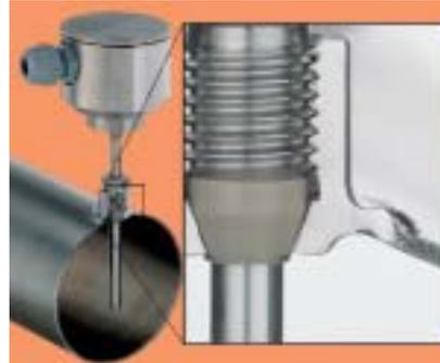
Clamp screwing with PEEK sealing washer sleeve LZE-NM in section view
