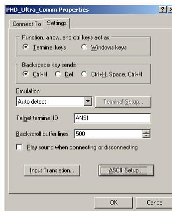
6. Choose ASCII Setup and select "Echo typed characters locally" then click OK to complete the setup.
