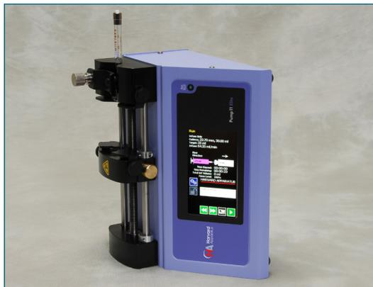
Advanced microstepping techniques are employed to further reduce the step angle to eliminate flow pulsation. The accuracy is 0.5% (0.35% for Pico Plus Elite). A wide dynamic flow range from 1.26 pl/min to 88.40 ml/min (0.54 pl/min to 11.70 ml/min for the Pico Plus Elite) can be programmed into the pump. Flow rates are selectable with user selected engineering units from ml,  $\mu$ l, nl, pl, and hours, minutes and seconds.
