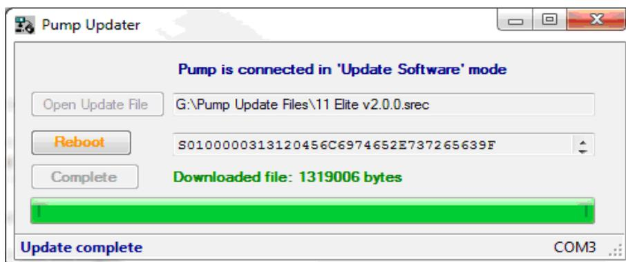
7. After the update is complete, press Reboot to power cycle the pump.
