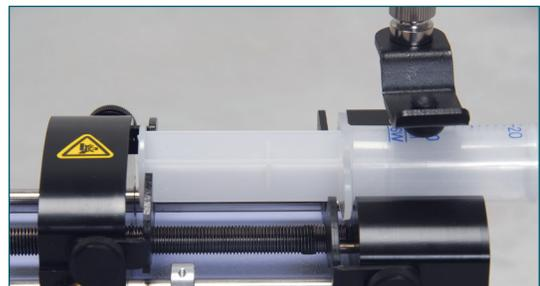
**CAUTION:** BE SURE MECHANICAL STOP COLLARS ARE POSITIONED PROPERLY TO PREVENT THE PLUNGER FROM BOTTOMING OUT ON GLASS SYRINGES.
