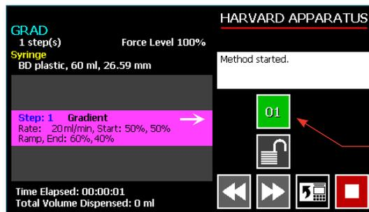
Pump Control button showing the satellite's address
