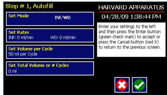
**TO SET UP/EDIT AN AUTOFILL CYCLING PROFILE:**
