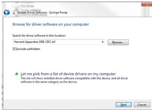
4. Click Browse and navigate to the pump drivers folder located on the CD supplied with the pump. Select the file Harvard Apparatus USB-CDC.inf. Make sure the Include Subfolders box is checked and then click Next.
