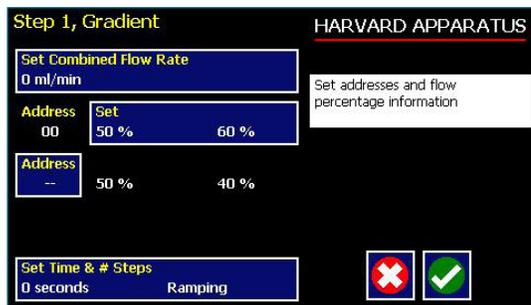
2. Enter the desired combined flow rate value for both pumps using the keypad or select the **Minimum Rate** or **Maximum Rate** button.
