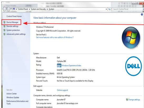
1. Connect the pump to the computer via USB. Open the control panel and select System and Security and then System. Click Device Manager on the left hand menu.
