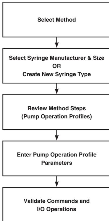
The software provides the user with a variety of prompts and warnings to help guide the setup of Methods. For example, if a pump Method incorporates steps that exceed the capacity of the defined syringe, the system will prompt you that parameters are out-of-range. The system also prompts users if required values are not entered.
