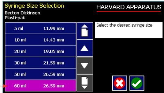
Press to enter the inside diameter of the syringe
