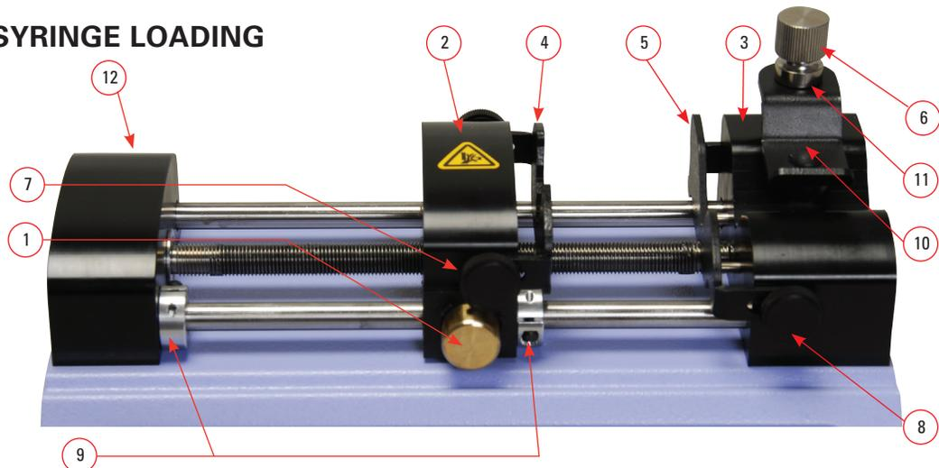
The Pump 11 Elite Series can accommodate up to two syringes. Depending on the mechanism, any type of syringe, glass, plastic or stainless steel can be used. The Pump 11 Elite can accommodate from 0.5 µl to 60 ml single syringe and 0.5 µl to 10 ml dual syringe. The syringe barrel clamp should be flipped for syringes smaller than 30 ml. For syringes larger than 30 ml the syringe clamp should be used as shown.
