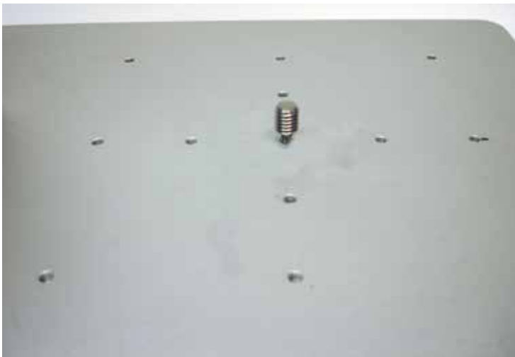
The LTCM-100 comes standard with the expanded work table. The work table has 13 pre-drilled, #10-32 threaded holes for mounting fixtures and grip sets. The optional expanded work table for the LTCM-500 has 13 pre-drilled 1/4-28 holes.
