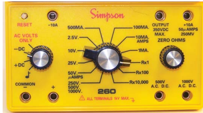
Figure 4-12. Jack and Switch Positions for Measuring Resistance
