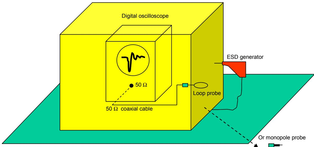
**Figure D.5 – Example of test setup to measure radiated ESD fields**
