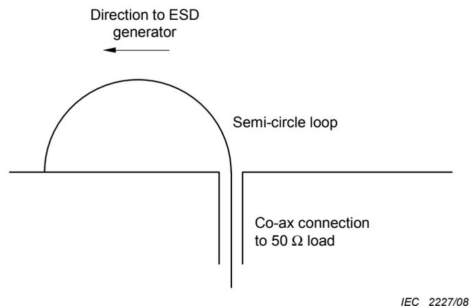
**Figure D.3 – Semi-circle loop on the ground plane**
