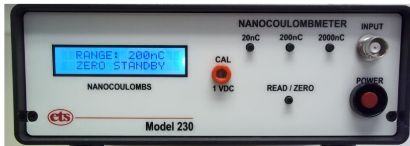
Figure 4.1: Model 230 Nanocoulombmeter front panel
