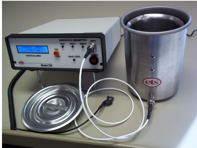
Figure 6.1: Faraday cup connections
