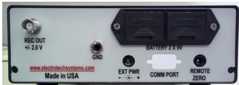
Figure 4.2: Model 230 Nanocoulombmeter rear panel
