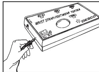
Figure 6. Installing ground cord to "footplate" jack.
