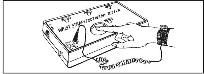
Figure 5. Testing of wrist strap grounding assemblies.
