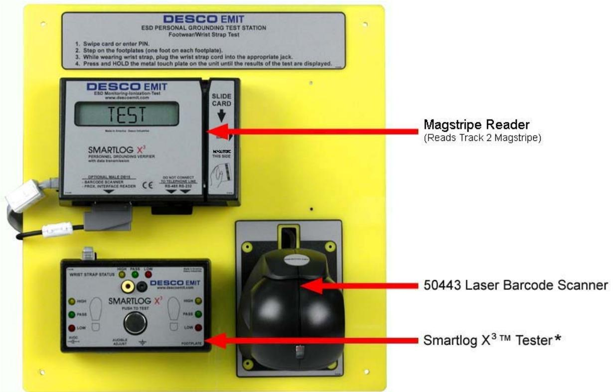
\*New Feature: Internal switch added to allow user to test only wrist strap or footwear.
