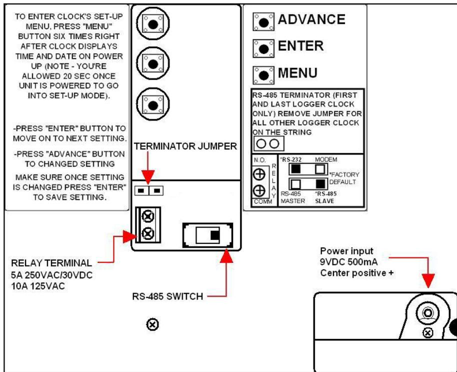
Figure 3. Back-side of SmartLog X<sup>3</sup>™ plate
