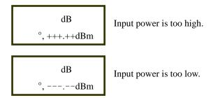
If MEAS? or READ? query command is executed in the remote operation when the input power is too high or too low, the instrument generates the device dependent error and saves it to the error queue. Refer to 3.3.Error codes for more specific descriptions. The return messages are all zero except the optical power value. The returned optical power is 100dBm when the input power is too high and -100dBm when the input power is too low.
