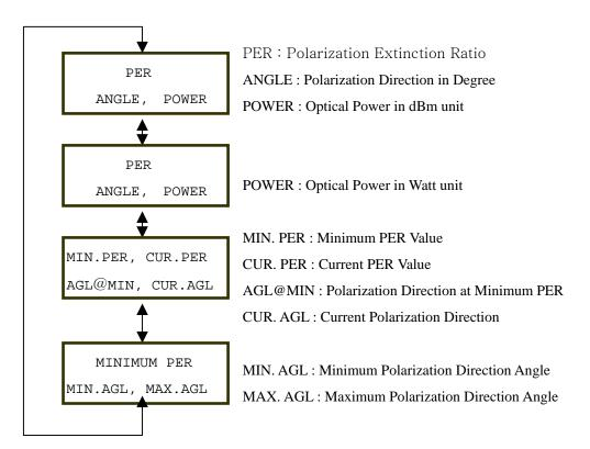
If [dBm/W] key is pressed during measurement, the display window will change to one of [PER / ANGLE / POWER] window.
