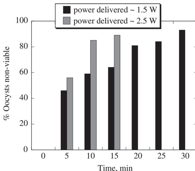
**Figure 1** Effect of sonication time and ultrasound power on the viability of *Cryptosporidium* oocysts (15–20°C; pH 7.4)
