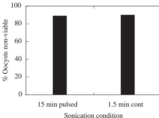
**Figure 2** Effect of continuous sonication on the deactivation efficiency of *Cryptosporidium* oocysts (power delivered ~2.5 W)
