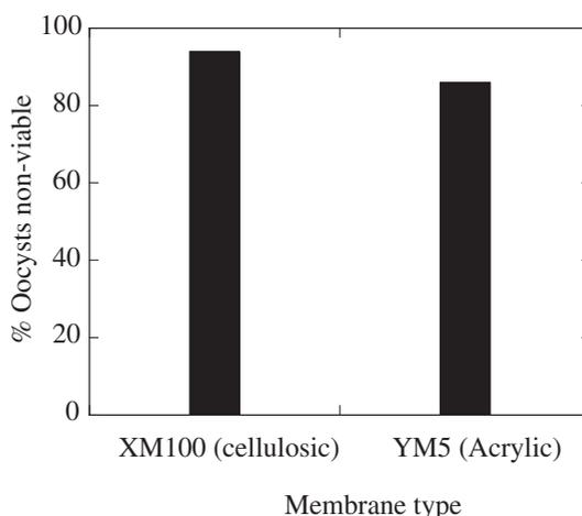
**Figure 4** Deactivation by 15 min sonication (pulsed; 1/10 duty cycle;  $\sim 1.5$  W power delivery setting) of *Cryptosporidium* oocysts following ultrafiltration and redispersion
