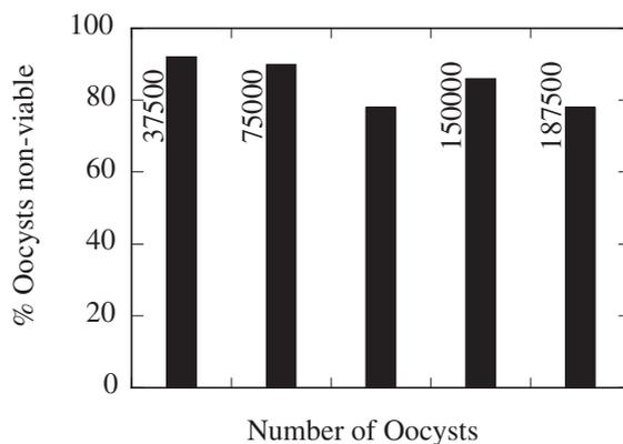
**Figure 3** Effect of variation of oocyst numbers on deactivation after 15min sonication (1/10 duty cycle) at a power delivery setting of  $\sim 2.5$  W (the numbers indicated in the figure correspond to the total number of oocysts present in each solution)
