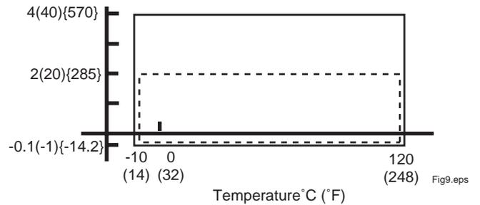
NOTE: This limits show maximum allowable fluid pressure for Flow Tube it self. Further fluid pressure should also be limited according to flange rating.
