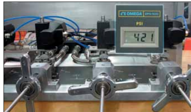
Probes are subjected to a leak test at the welded thermocouple junction (hot end) with a pressurization greater than 2.5 MPa (362 psi).
