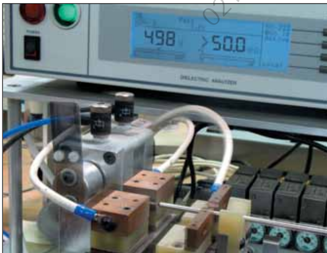
To pass the IR test according to ASTM specs, OMEGA's BLMI probes must achieve at least a 1 GΩ reading. The unit under test scored 50 GΩ.
