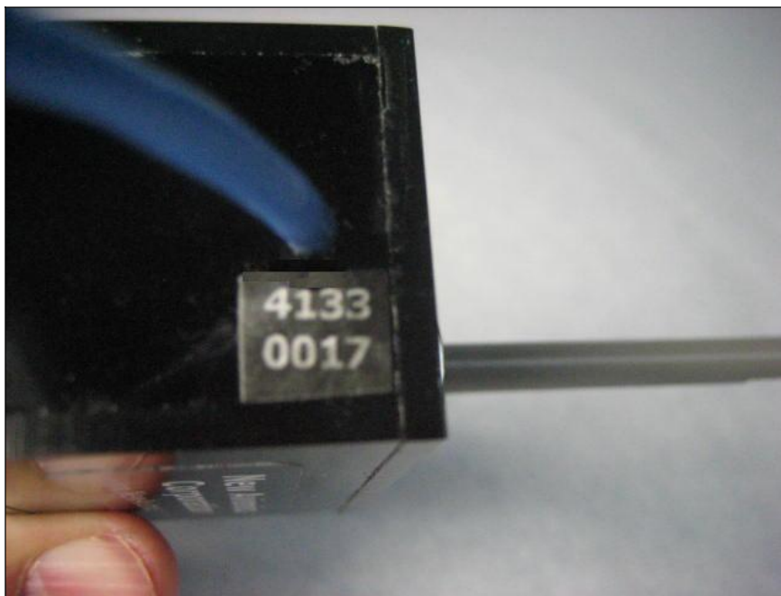
Figure 15 -- Serial number is located next to lightweight blue cable exit from aft bulkhead.
