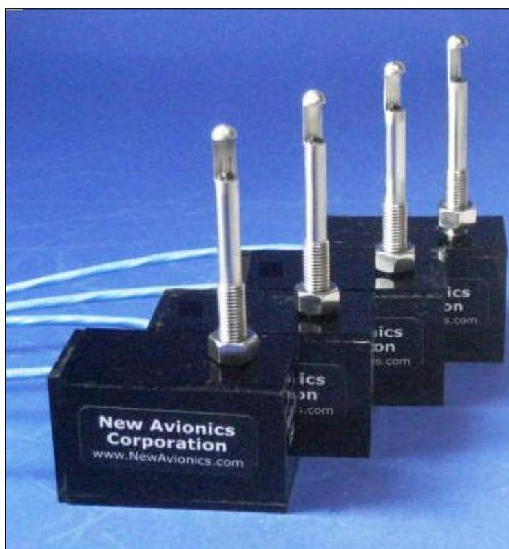
Figure 1 — Model 9732-STEEL aviation ice sensor is a commercial off-the-shelf, in-flight ice sensor. It monitors the optical characteristics of whatever substance is in contact with the optical surfaces of the sensor probe, either air (NO ICE) or water ice (ICE ALERT). Ambient wind stream blows liquid water away, but ICE molecules form and adhere to the optical surfaces for detection. Probe is tested by NASA, made of stainless steel, and is physically robust for use at subsonic airspeeds. Probe is set at 45 degrees to the airstream to protect the optics against airborne dust and particulates.
