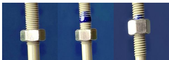
Figure 7 -- Installation nut is fixed with LOCTITE® 425™
