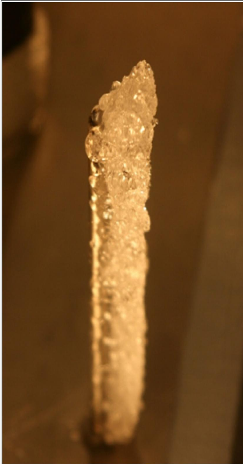
Figure 16 -- ice formation on sensor probe is by nature rough, imprecise, "fuzzy".
