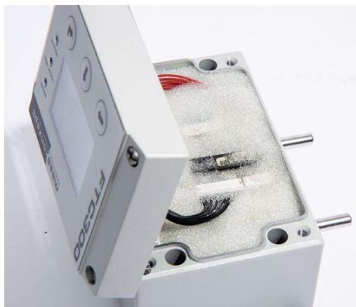
热导芯片有保护层 With Protection
