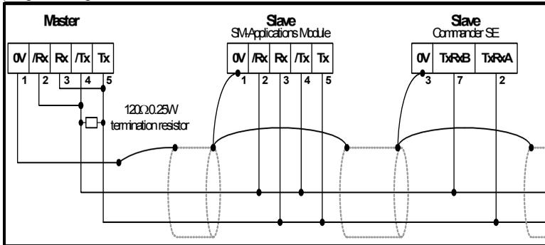
An EIA-RS232 to EIA-RS485 converter with “intelligent transceiver switching” (also known as “magic” EIA-RS485 converters) is required to allow a standard PC serial port to communicate with a 2 wire EIA-RS485 network. An example of a “magic” converter is the MA485F converter from Amplicon.
