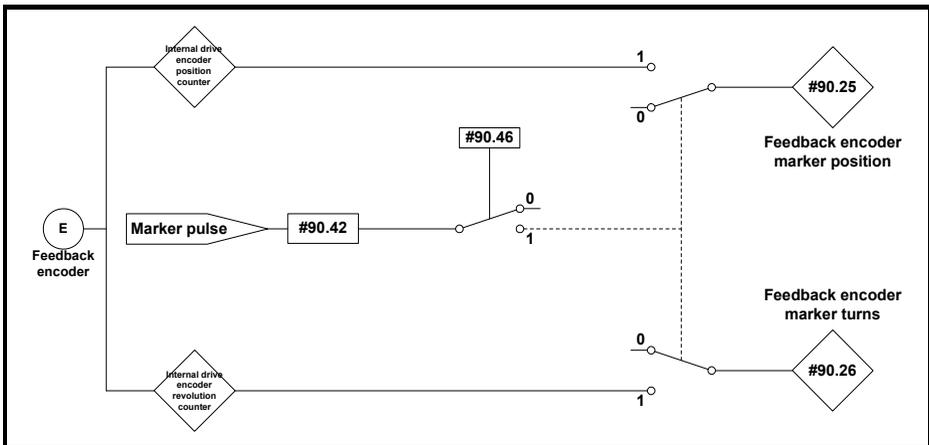
The marker position is cached into Pr **90.25** and the marker revolution counter is cached into Pr **90.26**.
