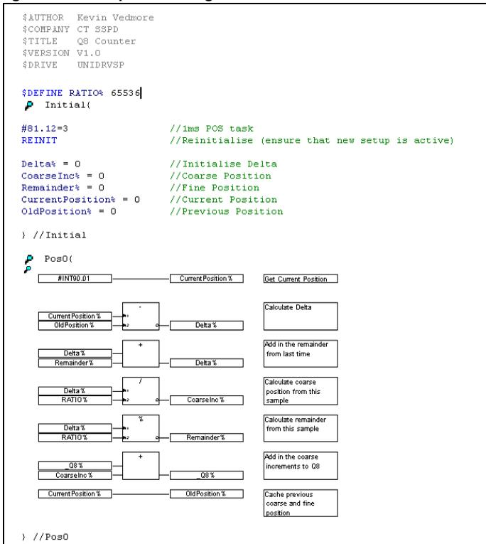
This program will take the positional feedback information from the drive (which is scaled to  $2^{32}/\text{rev}$ ), work out the delta (which will be proportional to speed) and convert to encoder counts (based on a standard quadrature encoder) and add this to an accumulator.
