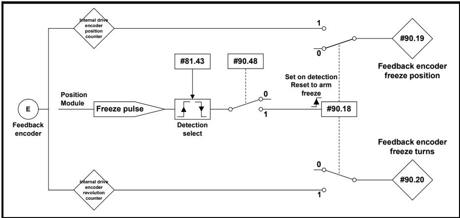
The encoder revolution counter is cached into Pr **90.19** and the encoder position is cached into Pr **90.20**.
