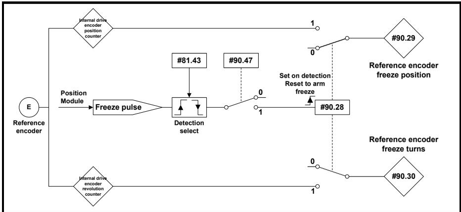
The encoder revolution counter is cached into parameter Pr **90.29** and the encoder position is cached into Pr **90.30**.
