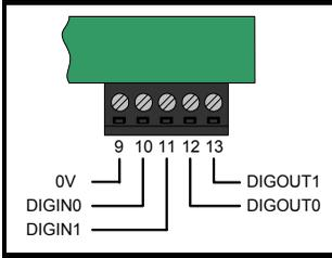
The SM-Applications, SM-Applications Plus and Digitax ST Plus are equipped with 2 digital inputs, known as DIGIN0 and DIGIN1, and 2 digital outputs, known as DIGOUT0 and DIGOUT1. These inputs and outputs can be read/controlled from the user program loaded into the SM-Applications Modules & Motion Processors .
