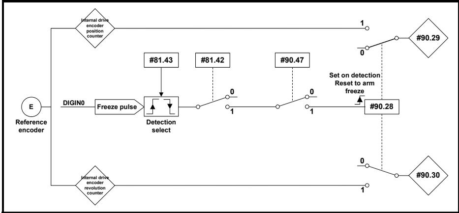
The encoder revolution counter is cached into Pr **90.30** and the encoder position is cached into Pr **90.29**.
