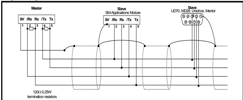
An EIA-RS232 to EIA-RS485 converter is required to allow a standard PC serial port to communicate with a 4 wire EIA-RS485 network.
