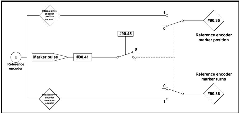
The marker position is cached into Pr **90.35** and the marker revolution counter is cached into Pr **90.36**.
