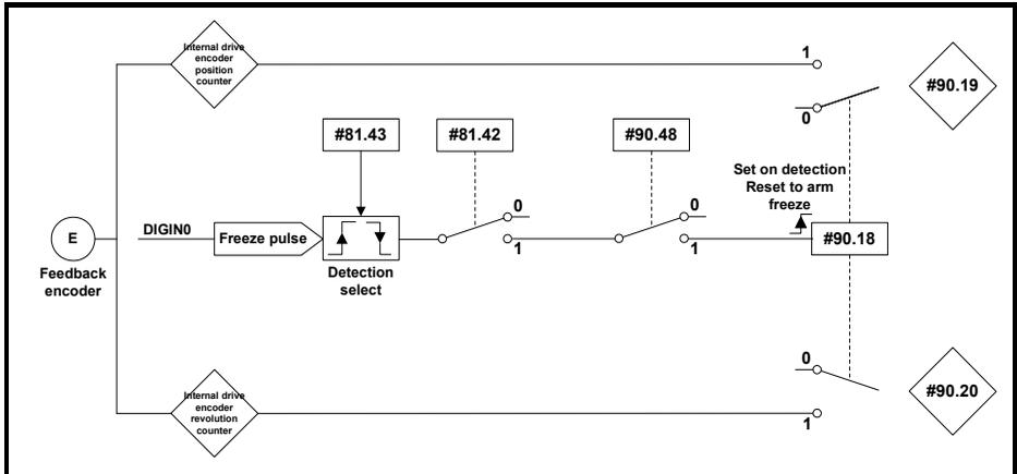
The encoder revolution counter is cached into parameter Pr **90.20** and the encoder position is cached into Pr **90.19**.
