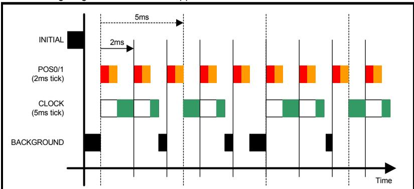
This shows the POS0 and POS1 tasks interrupting the CLOCK task which in turn interrupts the BACKGROUND task. As can be seen, this is quite a heavily loaded program since the background task is only executed once in a while. The processor free resource parameter Pr **81.04** can be used to determine how heavily loaded the Second Processor is.
