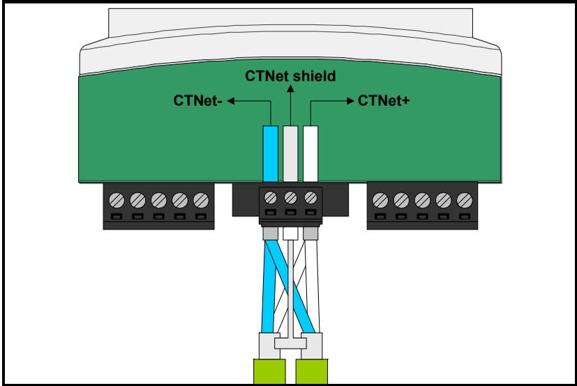
The shields of both cables should be twisted together and connected into the centre terminal of the 3-way terminal block. This “pigtail” should be kept as short as possible. This design guarantees shield continuity.
