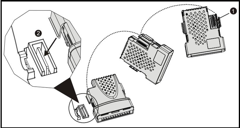
The Solutions Module connector is located on the underside of the module (1). Push this into the Solutions Module slot located on the drive until it clicks into place (2). Note that some drives require a protective tab to be removed from the Solutions Module slot. For further information, refer to the appropriate drive manual.
