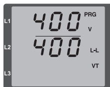
Fig. Programming mode Voltage transformer The primary and secondary currents can be changed using buttons 1 and 2 (cf. page 41).
