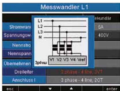
Fig.: Example for the configuration of current measurement via 3 current transformers in a three-phase 4-wire network on the UMG 509 display
