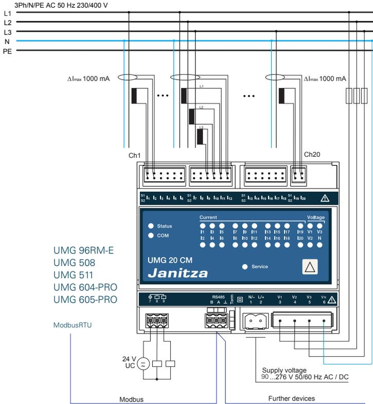
Recommendation: The bus should not contain more than 10 devices, type UMG 20CM if several UMG 20CM measuring channels are used. If the APP "20CM-Webmonitor" is used, the number is limited to 5 devices due to the APP management).
