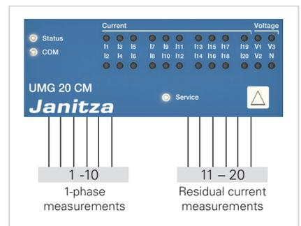
Fig.: 10 single-phase operational current measurements, 10 single-phase residual current measurements,
