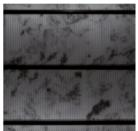
At wavelengths above 1100 nm silicon becomes transparent. Thus, SWIR cameras are perfect for analyzing metallization and electrical contact errors on the backside of wafers.
