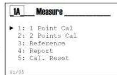
**校准步骤****校准菜单测量 (菜单 1A)**
