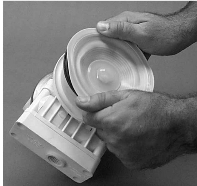
Step 10. Figure 10 Using an adjustable wrench, or by rotating the diaphragm by hand, remove the diaphragm assembly from the center section.
