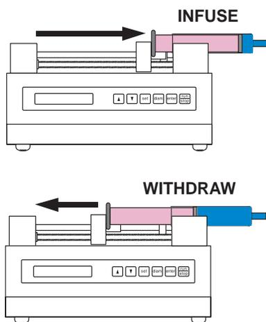
A motor driven threaded rod (lead screw) slowly turns, moving the plunger of the syringe in, and pushing the fluid out. Reversing the direction of the motor allows for withdrawal of fluids.
