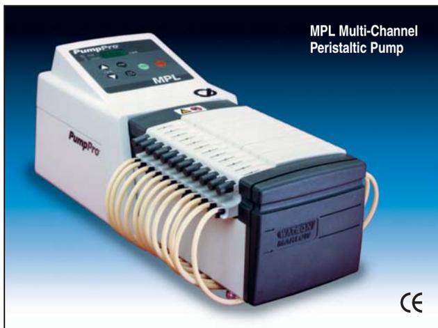
A 25 pin D-sub connector provides access to the external control features of the Manual/Analog pump. Through this connector the user can control pump speed and direction as well as perform start and stop functions. Pump speed can be regulated using either an external voltage (0 to 30 V) or current (0 to 30 mA) source. Additionally, pump operation and speed can be monitored through the 25 pin connector.
