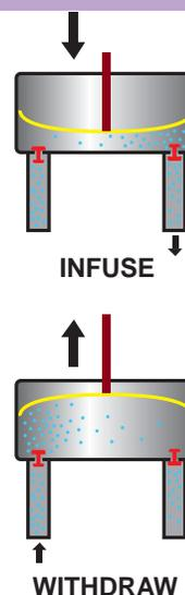
The red rod shown in this drawing is moved by a motor or solenoid. It pushes the diaphragm in and a spring forces it back out.
