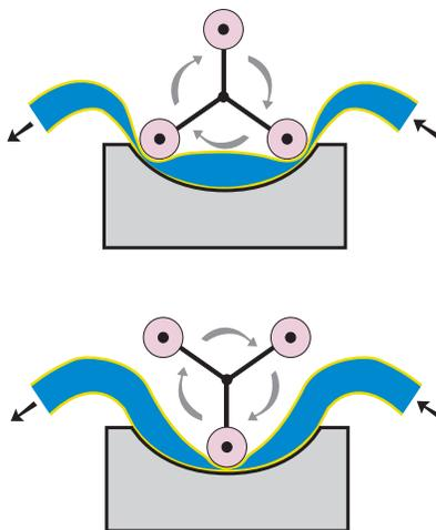
In this example three rollers on rotating arms pinch the tube against an arc and push the fluid along. There are usually three or four sets of rollers.
