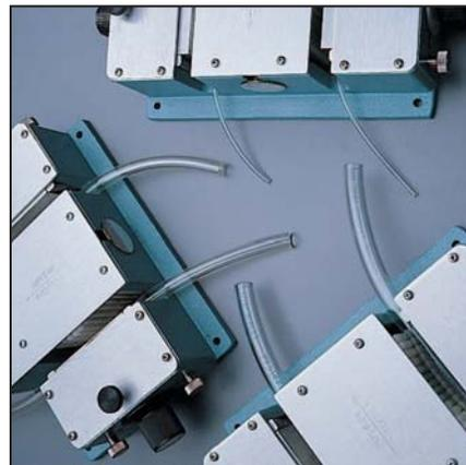
Adjusting the pumping channel for any size tubing from micro to 12.7 mm (1/2 in) is a simple process. Lay the tubing in the channel, release the pressure plate by the top thumb screws, screw the pressure plate forward until it properly grips the tubing, and lock the pressure plate in place.
