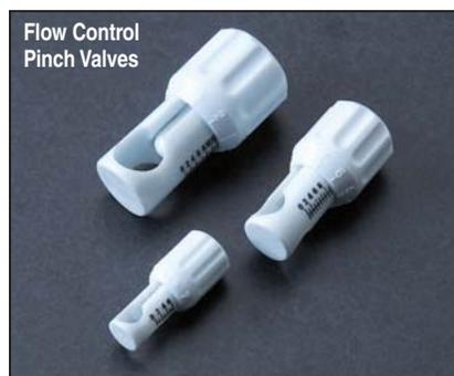
These variable tubing clamps work with tubing with OD of 5/32 to 1/2 inch. The micrometer dial offers easy resetting of clamping distance. Made of Delrin®.
