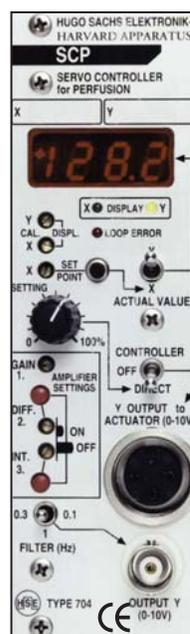
The PLUGSYS® plug-in unit "Servo Controller for Perfusion" (SCP) is used for the perfusion of organs and tissues using a peristaltic pump in the physiological and pharmacological laboratory. It is a conventional PID controller which operates to maintain either a constant perfusion pressure or a constant perfusion flow.
