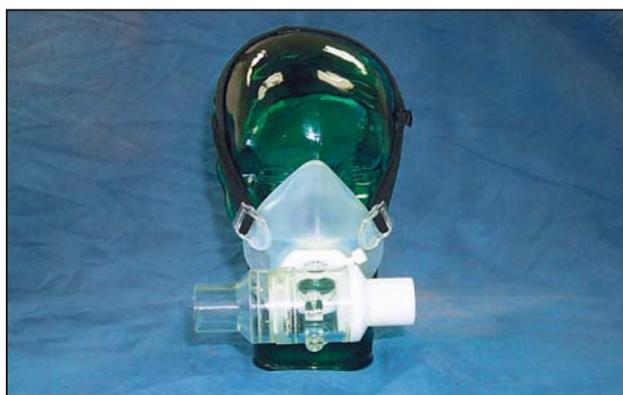
This adult facemask with integral non-rebreathing T valve is a high performance, very low dead space, low air flow resistance mask and valve; suitable for high air flow applications (e.g. exercise physiology). The AFT25 incorporates two gas sampling ports (female Luer) for interfacing with the AFT20 gas sampling kit. All ports are 35mm OD, 28mm ID.
