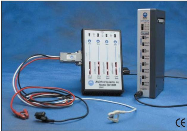
The TEL100C system offers a way to record data while subjects are mobile and/or physically distant (up to 60 meters) from the recording system. The TEL100C system includes a portable amplifier/transmitter, which converts up to four channels of data into a modulated data stream. This data stream travels over a single lightweight coaxial cable to the receiver module. The receiver module demodulates the data and sends it to the MP System for recording and analysis.
