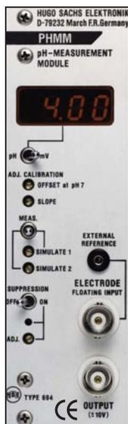
The HSE-HA pH Measurement module is used to measure pH with pH glass electrodes. The main application is continuously pH recording with the combination pH electrodes for measurement in biological fluids such as perfusate for isolated perfused organs. The input circuit of the module includes an isolation amplifier (potential separation between sensing electrode and circuit ground of the PLUGSYS measuring system) to avoid measurement errors due to ground loops and leakage currents.
