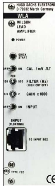
The WLA module Type 702 is used for capturing and amplifying unipolar ECG chest lead potentials after Wilson lead configuration in the PLUGSYS system. Up to 6 chest electrodes (V1 to V6) can be connected.
