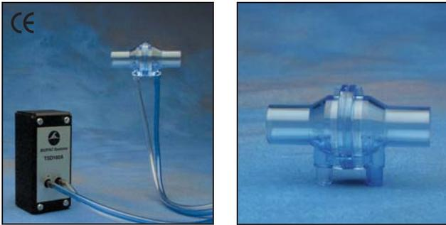
The TSD127 can perform a variety of pulmonary measurements relating to air flow, lung volume and expired gas analysis. The transducer includes a detachable flow head (RX127) for easy cleaning and sterilization. The TSD127 is intended for animal use and consists of a low flow, pneumotach air flow head (RX127) coupled to a precision, highly sensitive, differential pressure transducer (TSD160A). The TSD127 will connect directly to a breathing circuit or plethysmogram chamber.
