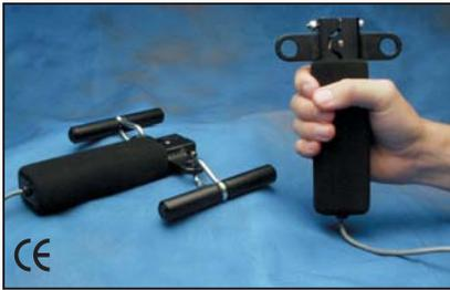
The TSD121C is an isometric dynamometer that measures a variety of gripping or pulling strengths for multiple muscle groups. The isometric design improves experiment repeatability and accuracy. Hand grip strength is easily recorded in pounds or kilograms force. Using the
