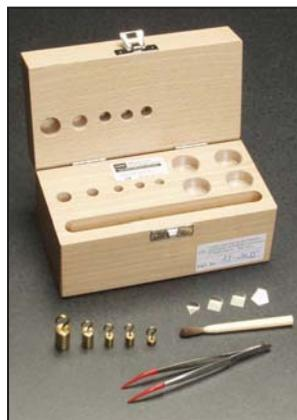
These gram calibration weights are precision weights use to calibrate preload on force transducers. The weights are made from polished brass. They are supplied in a wooden storage case with a pair of handling forceps and a cleaning brush. Nine weights are supplied. The 0.1, 0.2 and 0.5 gram size weights are flat metal pieces. The larger size weights have an integral hook. Class of accuracy M1 after OIML\*.
