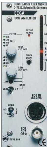
This module amplifies ECG signals. A floating input circuit is used to avoid hum and grounding problems. A bar graph display permits visualization of the ECG signal. The filters are for heart rates up to 1000 beats per minute. Both outputs can be used for recording on a chart recorder or for data acquisition. A square-wave signal generator with amplitudes of 0.3 mV and 1 mV is incorporated or calibration
