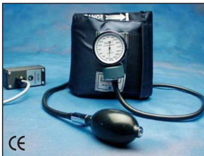
The TSD120 can measure systolic and diastolic blood pressure by the oscillometric or auscultatory (Korotkoff sounds) technique. The TSD120 includes an adjustable cuff (standard adult cuff: RX120D), pump bulb, pressure gauge and pressure transducer. The pressure transducer is attached to the cuff and connects to the DA100C
