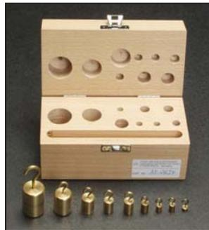
These NEWTON style calibration weights are precision weights use to calibrate force transducers. The weights are made from polished brass and have an integral hook. They are supplied in a wooden storage case. They are calibrated in Newtons at the standard acceleration of gravity  $g_n = 9.80665 \text{ m/s}^2$ . Nine weights are supplied. Class of accuracy M1.
