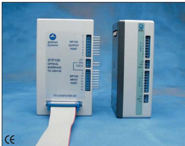
If you already have the SuperLab™ and the Digital I/O card with the Support Pack, you can interface to the MP System using the STP100 optical interface. The STP100 interface connects between the SuperLab™ Digital I/O card and the UIM100C module.
