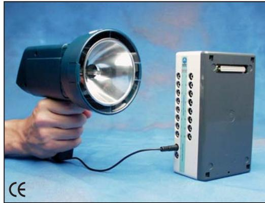
The TSD122 stroboscope connects directly to the UIM100C or STM100C module for single pass or averaging type visual evoked response applications. The stroboscope can be set up to either generate or respond to a TTL synchronizing signal for data acquisition. The TSD122 is battery-operated and will operate from zero to 12,000 flashes a minute. Cables are included for interfacing with the MP System.
