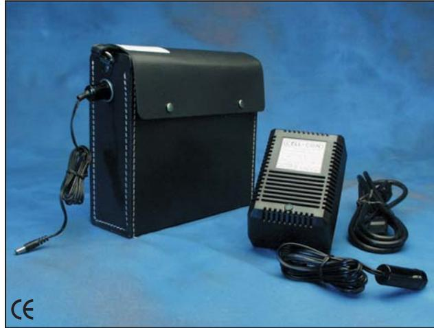
For portability, use this rechargeable battery pack and charger with your MP System. The maintenance-free battery pack is built into a carrying case with a shoulder strap. The fully charged battery will operate an MP System for a minimum of 16 hours. The BAT100 includes battery pack, universal recharger and all necessary cables.
