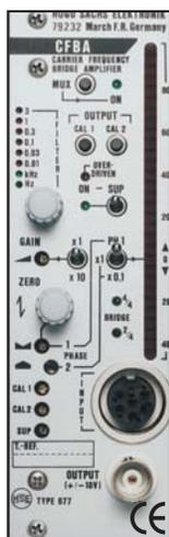
BS4 73-1602 Carrier Frequency Bridge Amplifier Module CFBA
