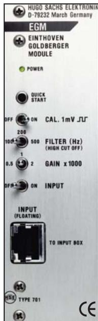
The EGM module is used for capturing and amplifying ECG signals after Einthoven and Goldberger lead configuration in the PLUGSYS system. It connects to 4 electrodes. This module has isolated input amplifiers in order to avoid hum interference.
