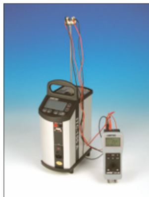
CSC200 as RTD input with an ITC
