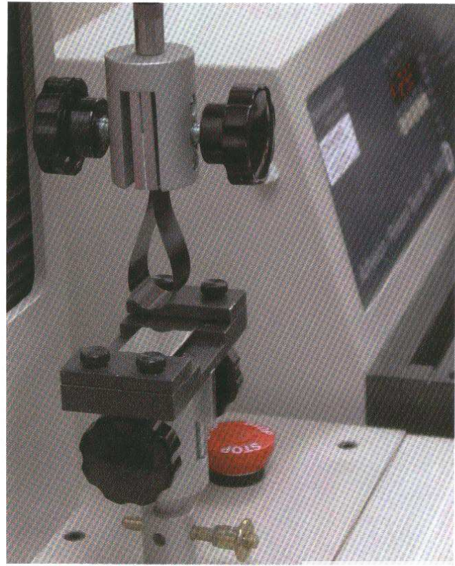
Figure 4. Tensile fixture mounted in tensile tester.
