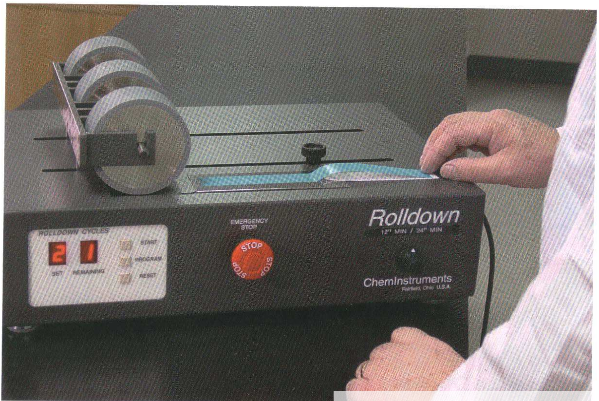
Figure 2. Mechanical roll down unit.
