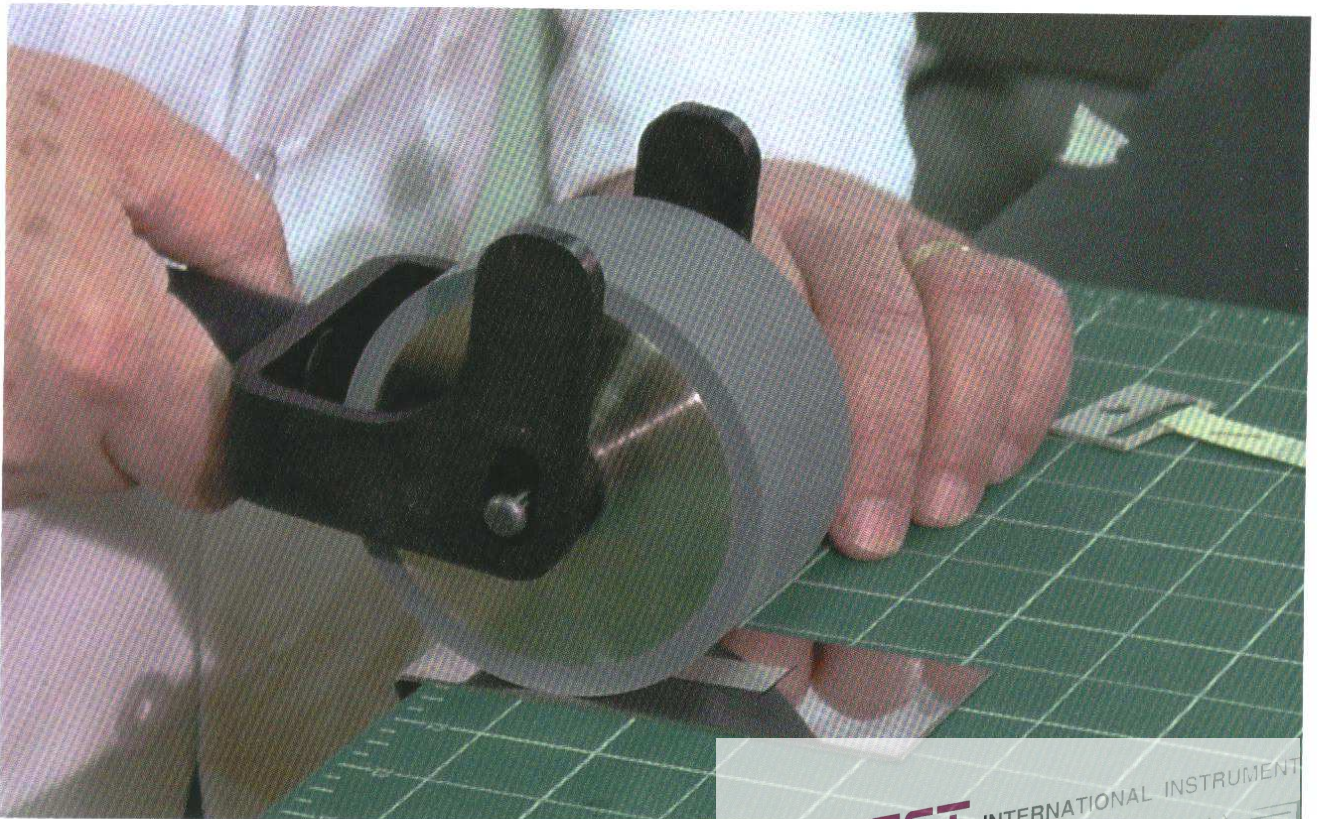
Figure 5. Sample preparation for shear adhesion hand roll down
