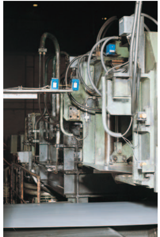
▲ Extreme operating conditions exist in steel making plants – the WT45 photoelectric proximity switch is ideal for many applications, such as detecting metal sheets before they are wound onto coils.
