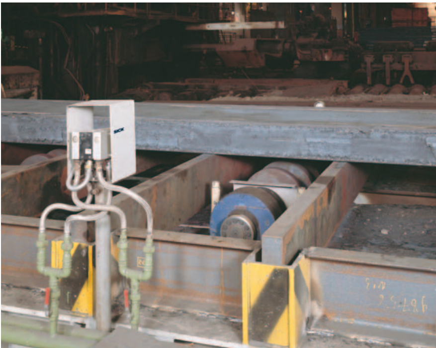
▲ Extreme operating conditions exist in steel making plants – the WT45 photoelectric proximity switch is ideal for many applications, such as detecting metal sheets before they are wound onto coils.
