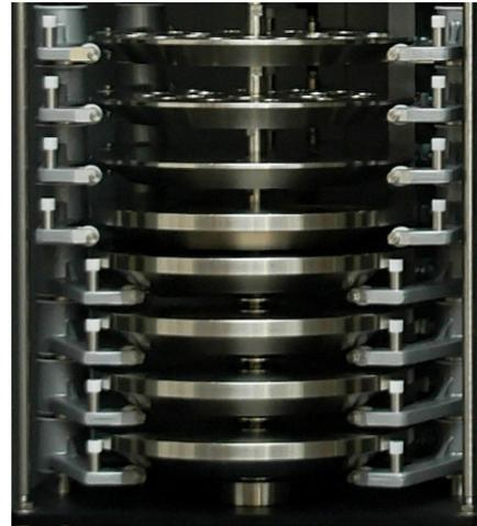
The main masses (from 2048 g up to 16384 g) are loaded / unloaded with three arms linked to a pneumatic actuator. All movement are user adjustable.
