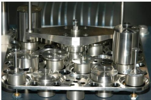
The small masses (from 0.1 g to 1024 g) are directly loaded / unloaded with a small actuator. The masses from 16 g up to 1024 g are composed of 2 masses of half weight (i.e. 32 g=2 masses of 16 g) and they are physically in opposed position to keep a good centring of the piston and not apply lateral perturbation force.
