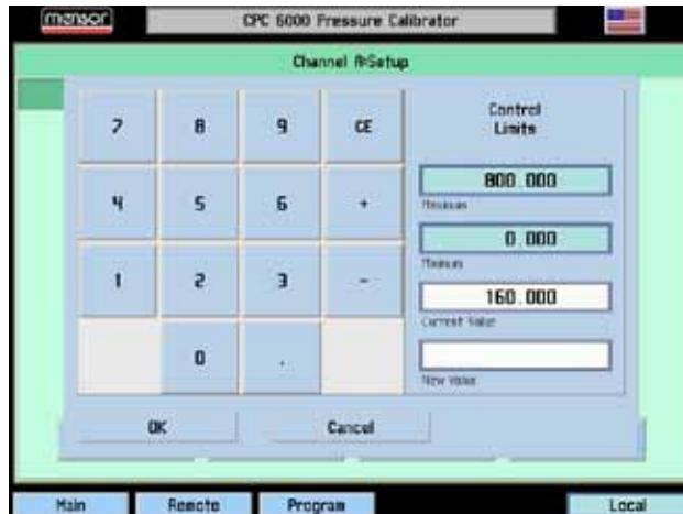
Figure 6.7.1B - Control Limits Window
