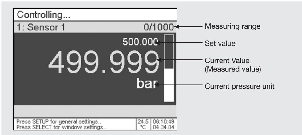
On the display of the CPC8000-H the set value and the current measured value (actual value) are clearly displayed. The colour of the measured value changes from white to green immediately the controller achieves the set value in accordance with the accuracy class. Decimal places can be increased or decreased via the menu (altogether up to 7 full digits can be displayed).
