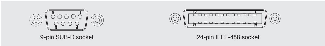
For PC driven operations, e.g. automatic calibration procedures, the required set value can also be set via the digital interface. For this, the high-pressure controller has an RS-232 and an IEEE-488.2 interface on the back. The interface instruction set is based on standard SCPI commands, which can be communicated by one's own program or through standard software e.g.: LabView®.
