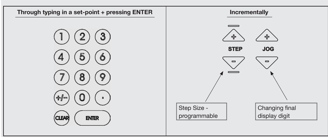
A pressure (set value) can simply be input via the keypad and confirmed by pressing the enter key. Optionally, the pressure can also be changed incrementally using the STEP and JOG buttons.
