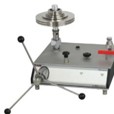
High-pressure pressure balance model CPB5000HP
