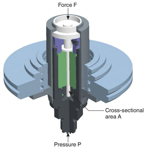
**Piston cylinder system model CPS5000**
