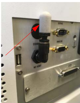
Figure 8-1 Dry Nitrogen Vent
