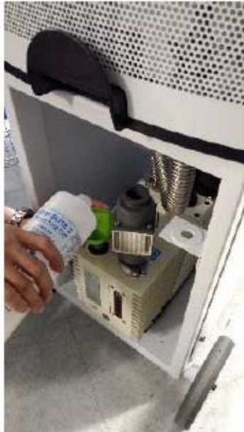
Figure 1-12 Mobile Unit Oil Fill
