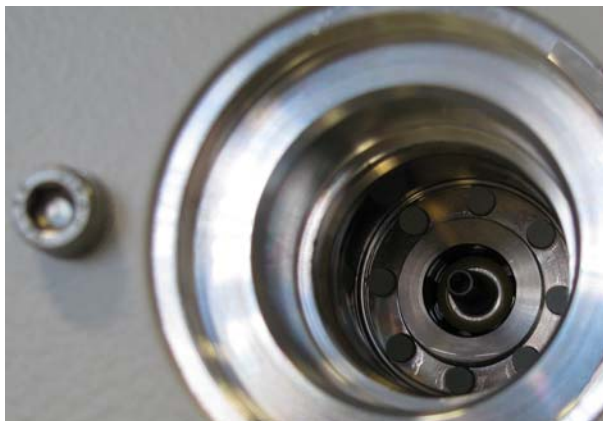
Fig. 50: Porex rods of the operating fluid reservoir
