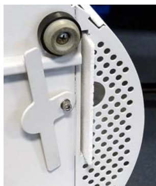
Fig. 47: Air filter in the air filter duct
