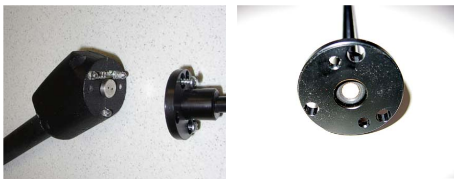
Fig. 55: Sinter filter in the sniffer handle
