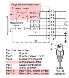
Connect the sensor cable to the gauge and the control-
