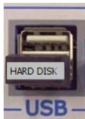
The USB storage key must be ALWAYS connected to the bottom port (see picture below). This USB key works as the inner memory of the system. It contains the collected data and the protocols.
