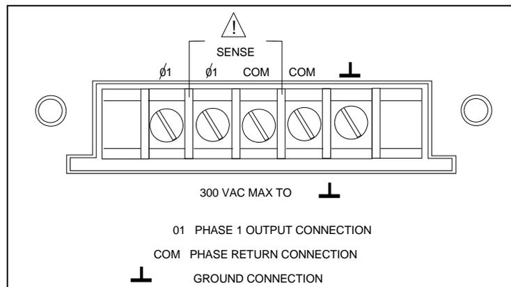
**Figure 2-4. Output Connections**
