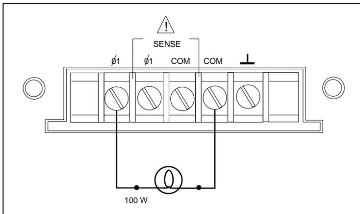
Figure 3-1.Verification Connections
