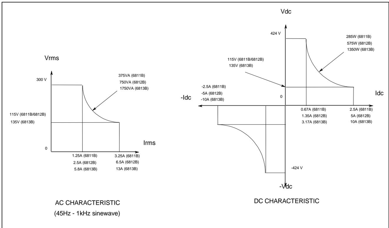
Figure 1-2. Steady-state Output Characteristic (in real-time mode)
