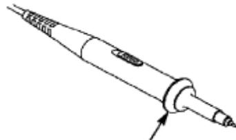
Figure 0-5: Finger Safety Ring of the Probe
