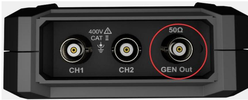
Figure 5-1: Generator Output Ports
