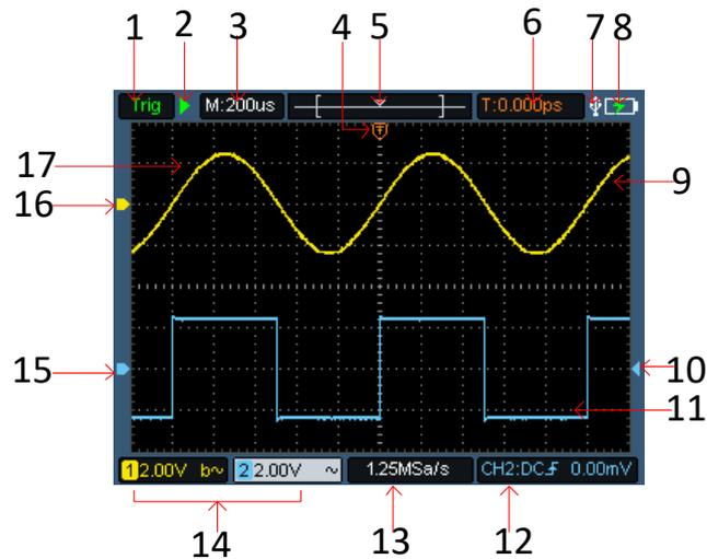
Figure 5: Oscilloscope Interface
