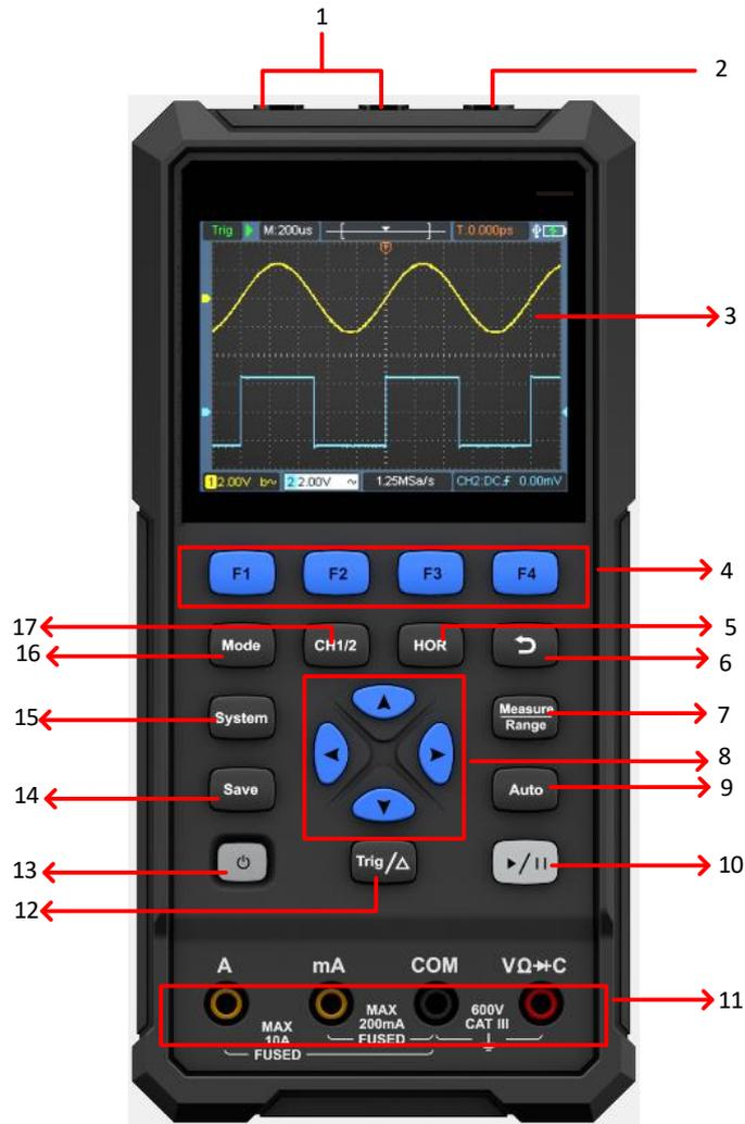
Figure 4: Front Panel of the Oscilloscope
