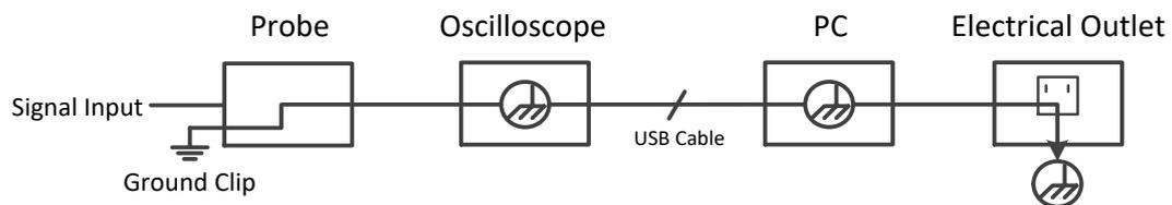
When the oscilloscope is AC powered by adapter or connected with AC
