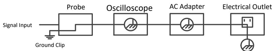
Schematic diagram of internal ground connection when oscilloscope is connected with computer through the port:
