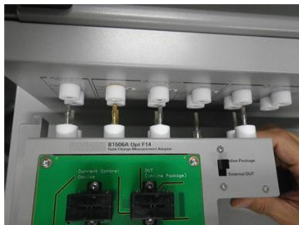
Figure 5-6 Attaching the Qg adapter to B1506A test fixture.
