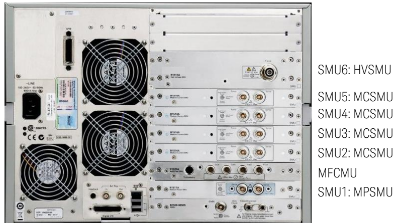
Figure 1-1. Module configuration of B1506A H-51 and H71.
