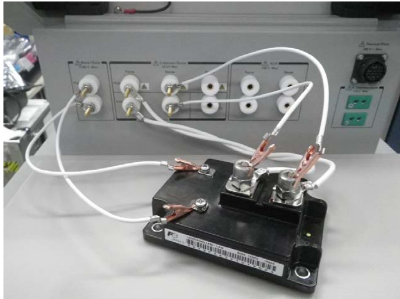
Figure 5-35 Setup using the output resistance of the UHCU as a resistive load.
