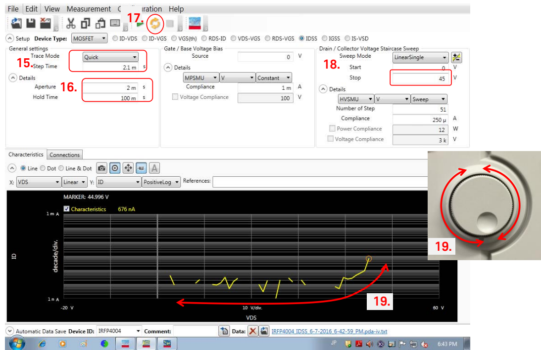
Figure 3-28 Interactive drain leakage current measurement
