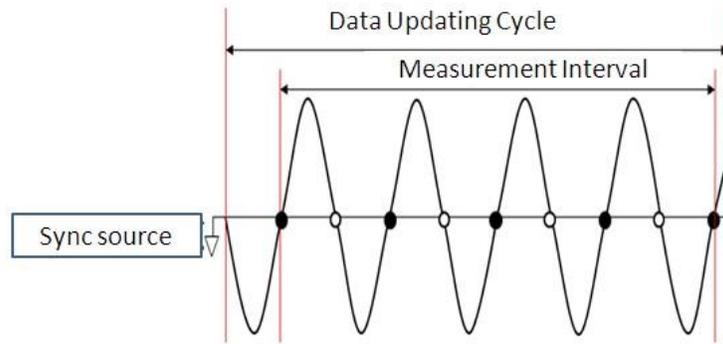
Figure 3.1: Measurement Timing
