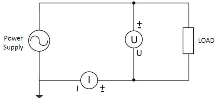
Figure 1.4: Low Current Wiring Setup
