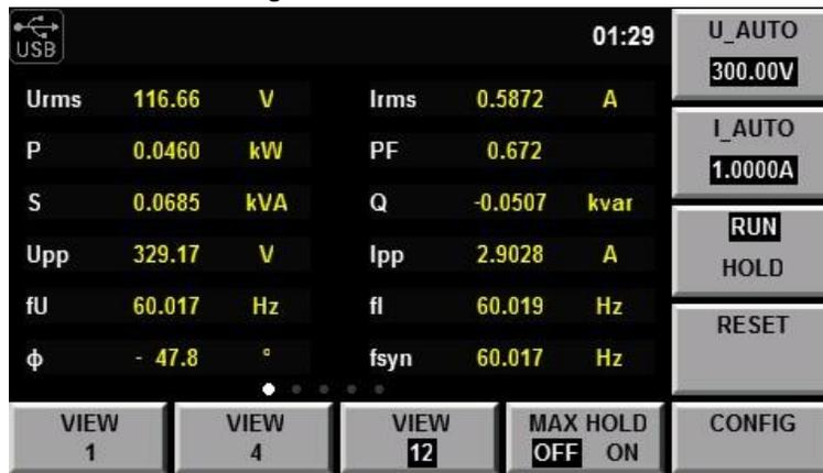
Figure 4.3: 12 main measurements
