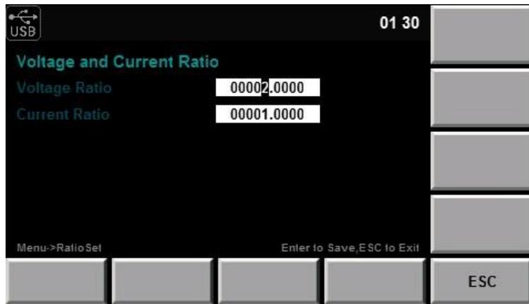
Figure 2.4: Ratio Setup Menu
