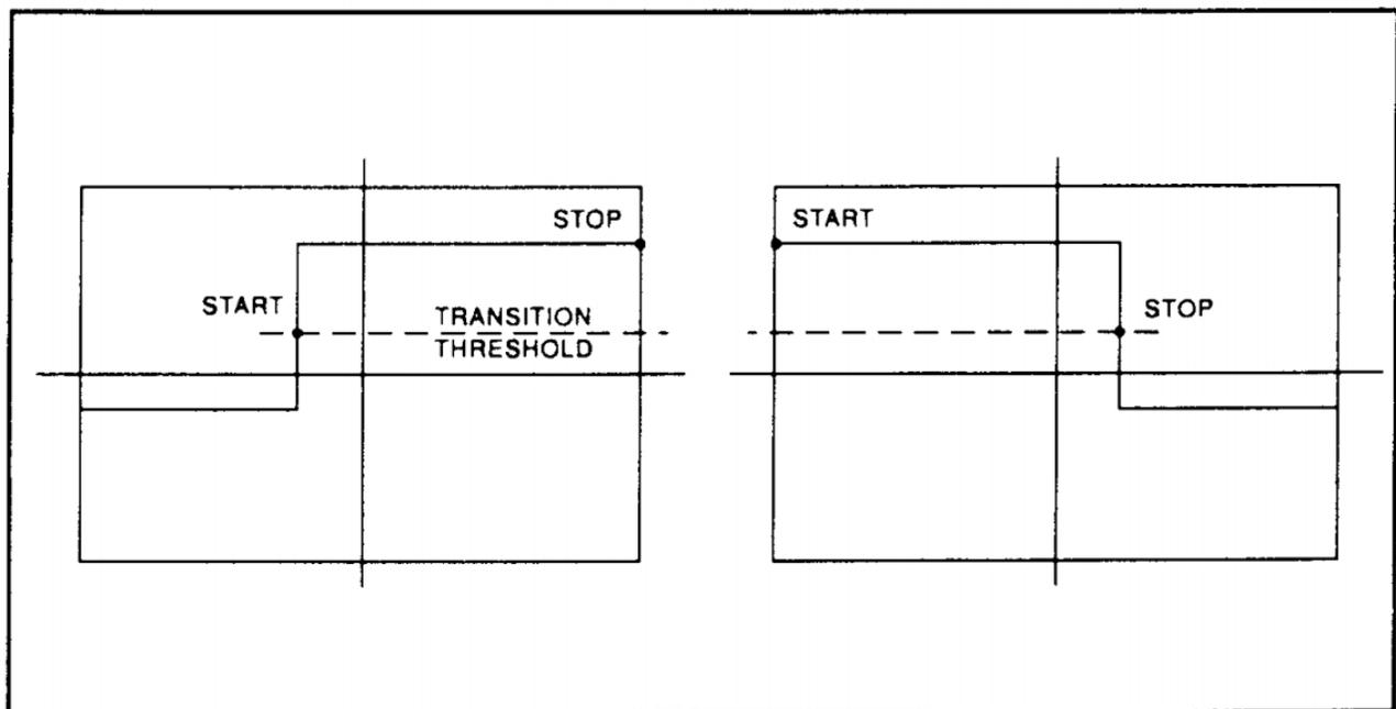
**Figure 5.5** Step Waveforms
