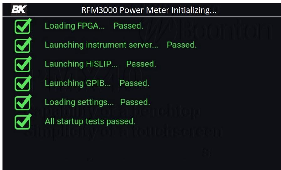
Figure 6.1 Self-Test Results
