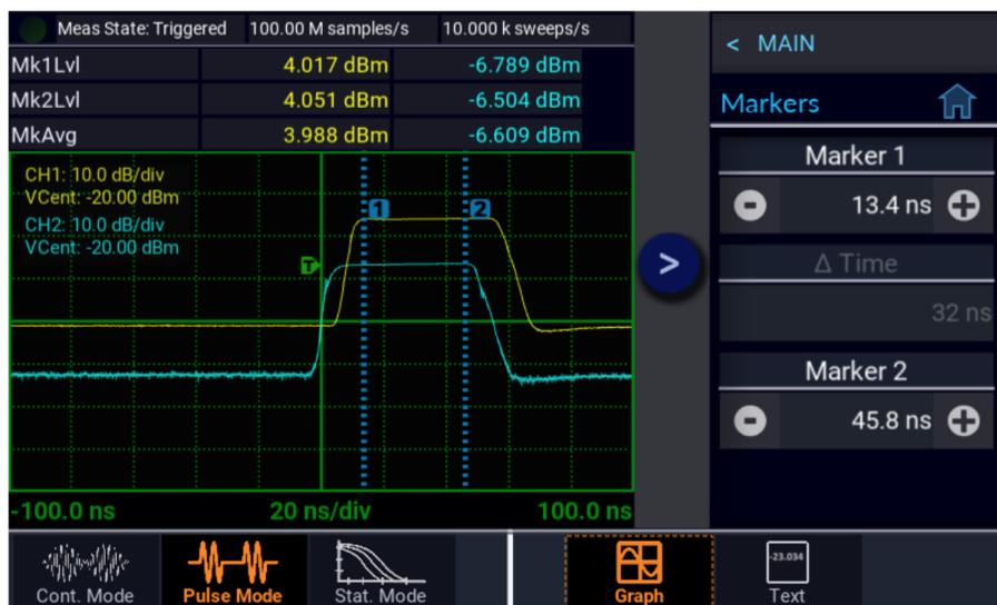
Figure 3.2 Marker Measurements
