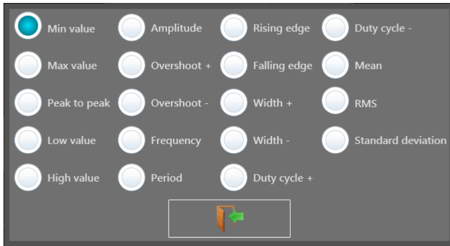
Figure 4.7 F(t) Channel Math Functions Dialog
