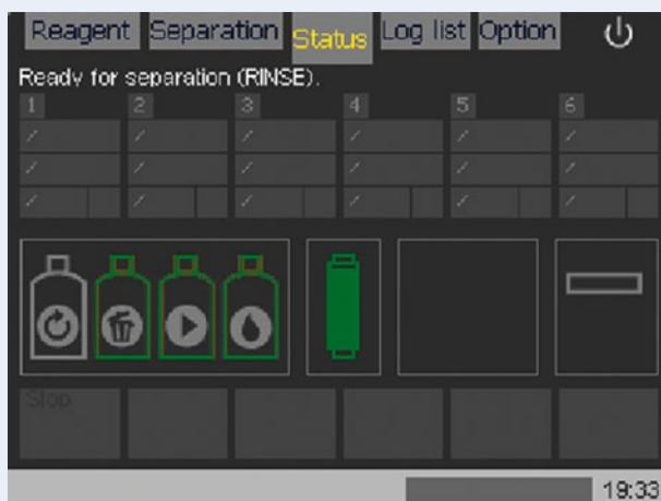
Figure 7: Status menu screen will display instrument status, fluid container status, and monitor column status.
