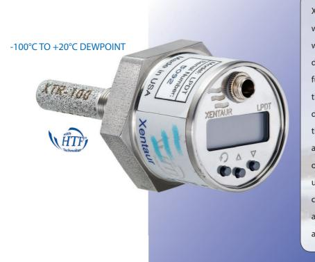
Xentaur's Model LPDT is the world's smallest loop powered (2wire) dewpoint transmitter with a display. The compact LPDT is a fully functional instrument operated through a miniature custom LCD display and three push buttons, using the same user friendly interface of all Xentaur hygrometers. The analog output is linear to the engineering units selected for display and is user configurable. A weatherproof cap is available for outdoor NEMA 4X (IP65) applications.
