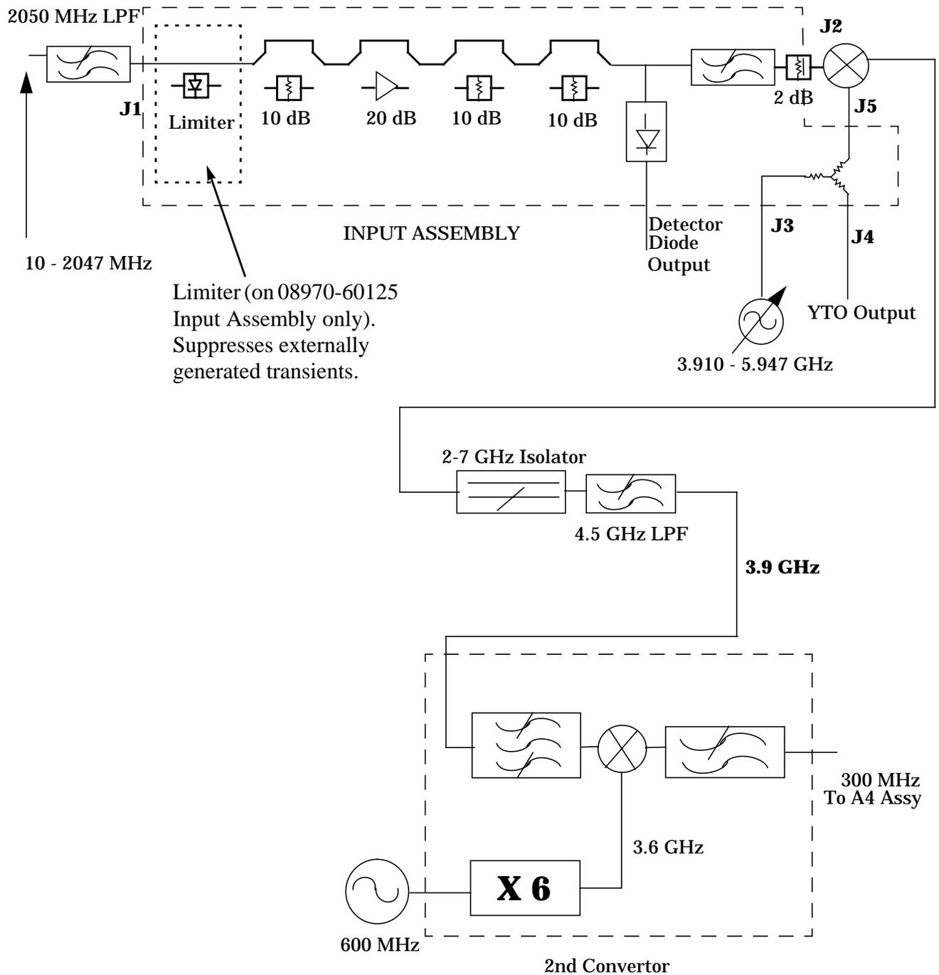
**Figure 1-3: Schematic Representation of Input Assembly**
