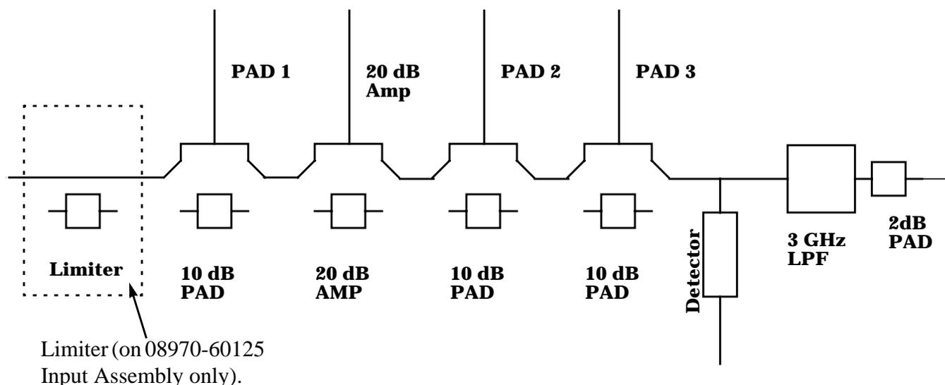
The easiest way to determine any problems with this section is to use a signal generator or sweeper which can cover the frequency range 10 MHz to 2047 MHz and can output -20 dBm.
