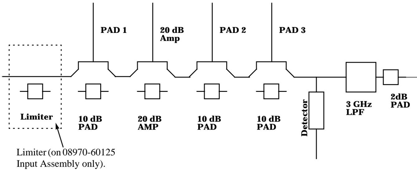
This is a schematic representation of the RF input assembly. The amplifier section and each and each of the attenuator sections are switchable by the control lines.
