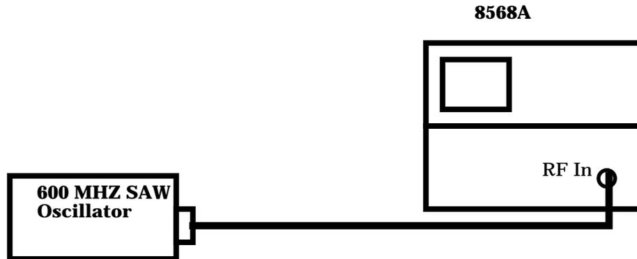
1. Disconnect the 600 MHz SAW Resonator from the second convertor 600 MHz input.
