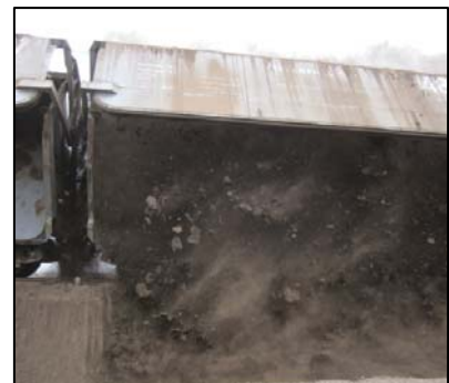
Cleaning from adhering ashes
