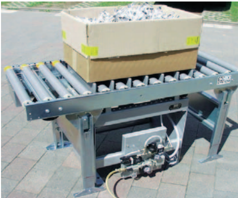
Compacting / levelling materials in a production line with a vibrating table
