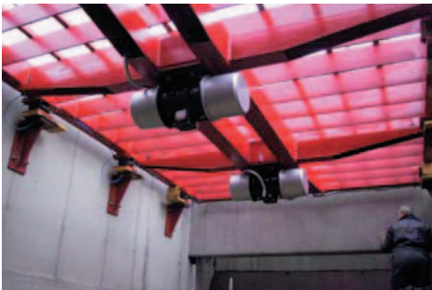
Sieving coarse bulk material with electric external vibrators
