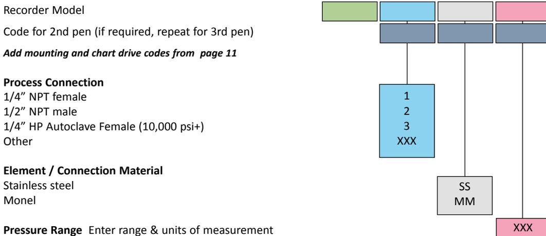
**Ordering Codes - Recorders fitted with Differential Pressure Systems**
