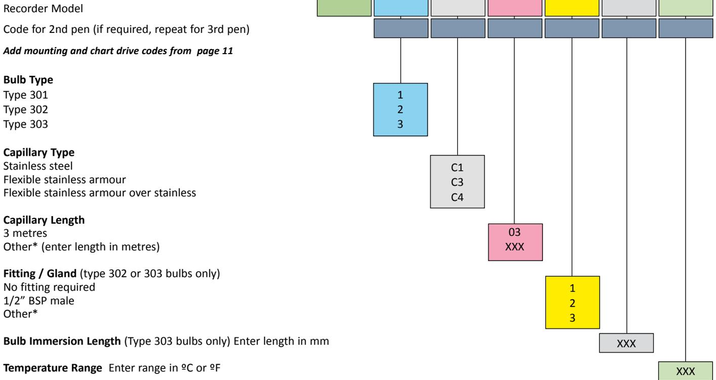
**Ordering Codes - Recorders fitted with Pressure Systems**
