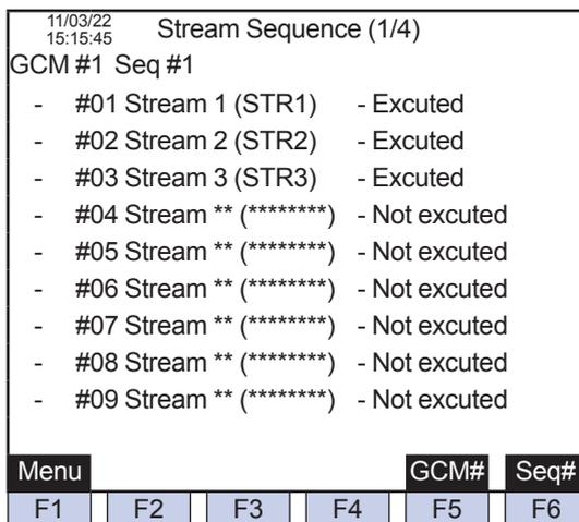
**Figure 1.21** An example of the stream sequence setting screen on the GC-HMI EtherLCD
