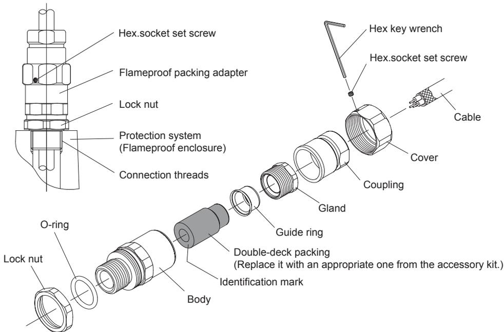
**Figure 2.13 Procedure for mounting a cable packing adapter for a protection system**
