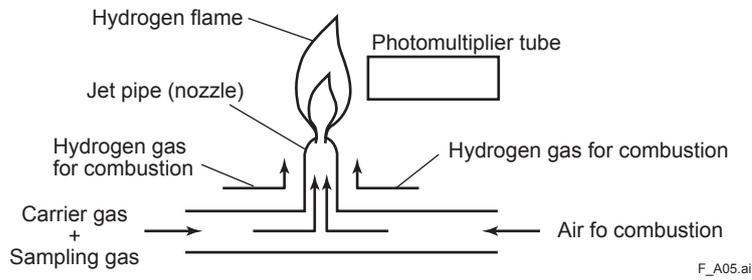
**Figure 5 Basic Configuration of Flame Photometric Detector**
