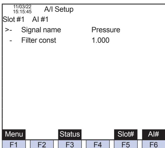
Figure 14 AI Setting Screen on GC-HMI EtherLCD
