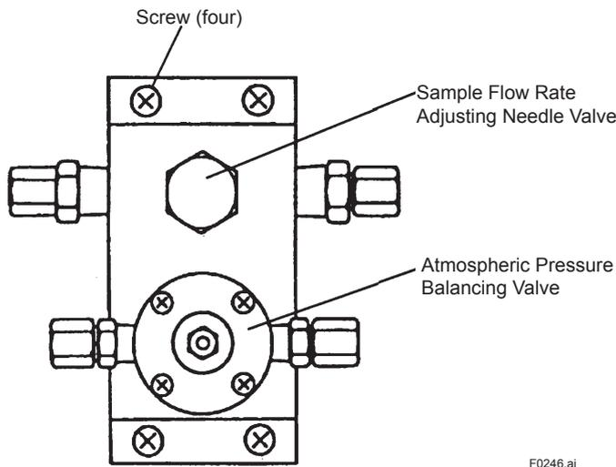
Figure 6.46 Atmospheric Pressure Balancing Valve and Sample Flow Rate Adjusting Needle Valve
