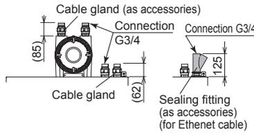
For FM-X (wiring connection: 3/4NPT)
