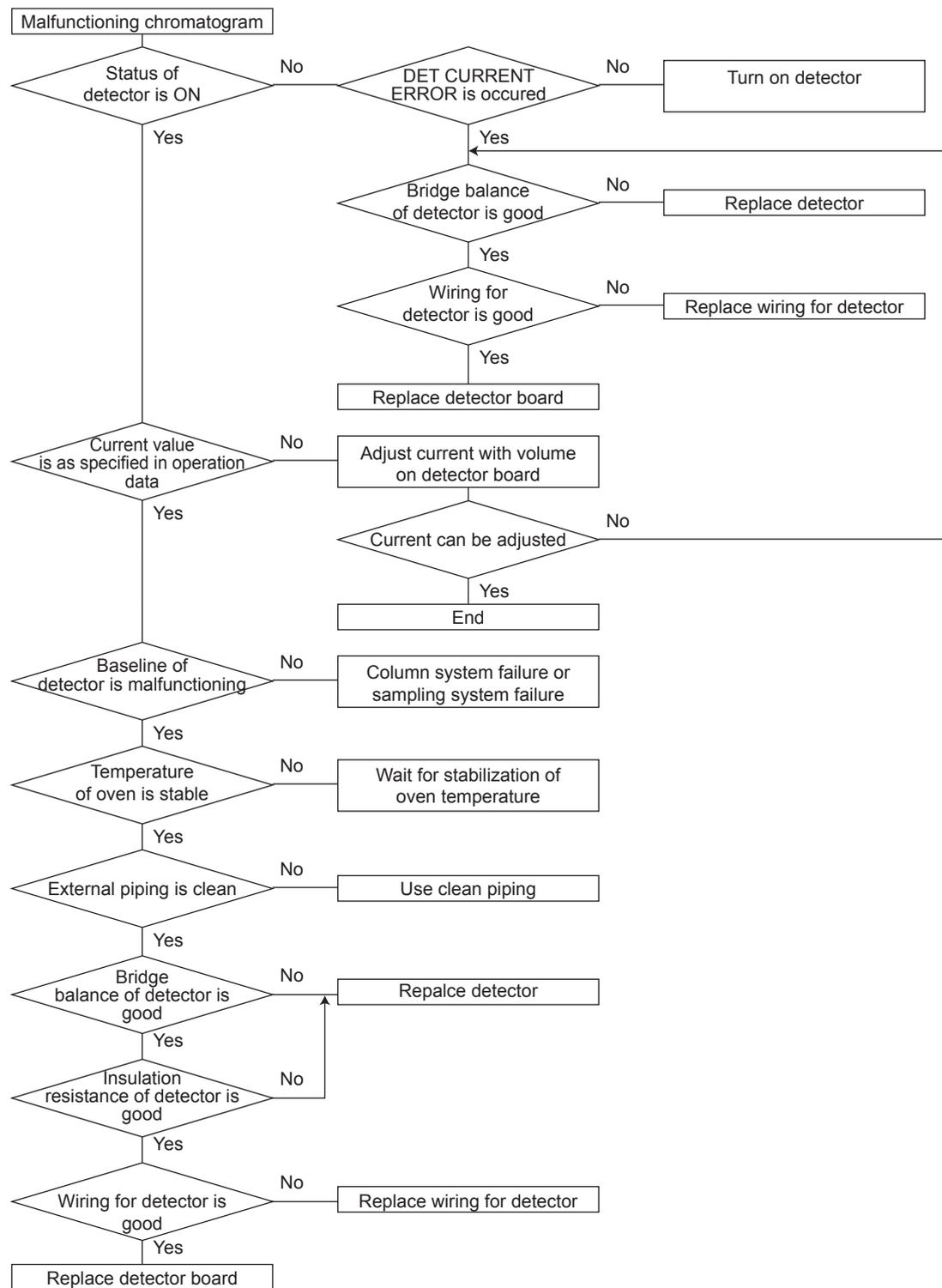
Figure 7.4 Troubleshooting Diagram for Malfunctioning Chromatogram (TCD)
