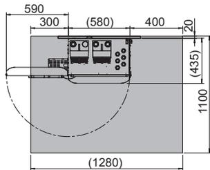
\*4: Required clearance needed for wiring.
