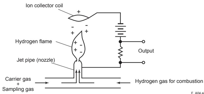
Figure 4 Fundamental Principle of Flame Ionization Detector
