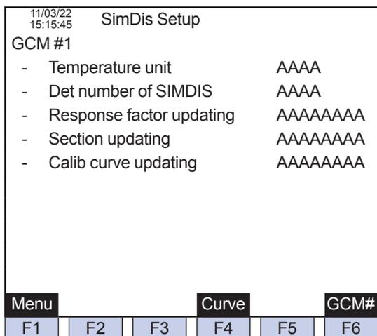
**Figure 5.140** Example of SimDis Setup screen
