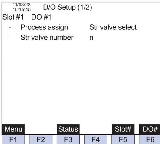
Figure 5.117 Example of DO setup screen (setting the Process assign to Str valve select)
