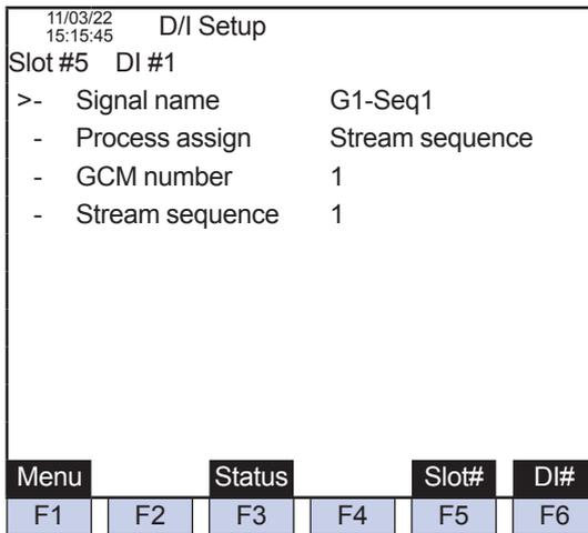
Figure 22 Process Specification: Stream Sequence (DI Setting Screen on GC-HMI EtherLCD)
