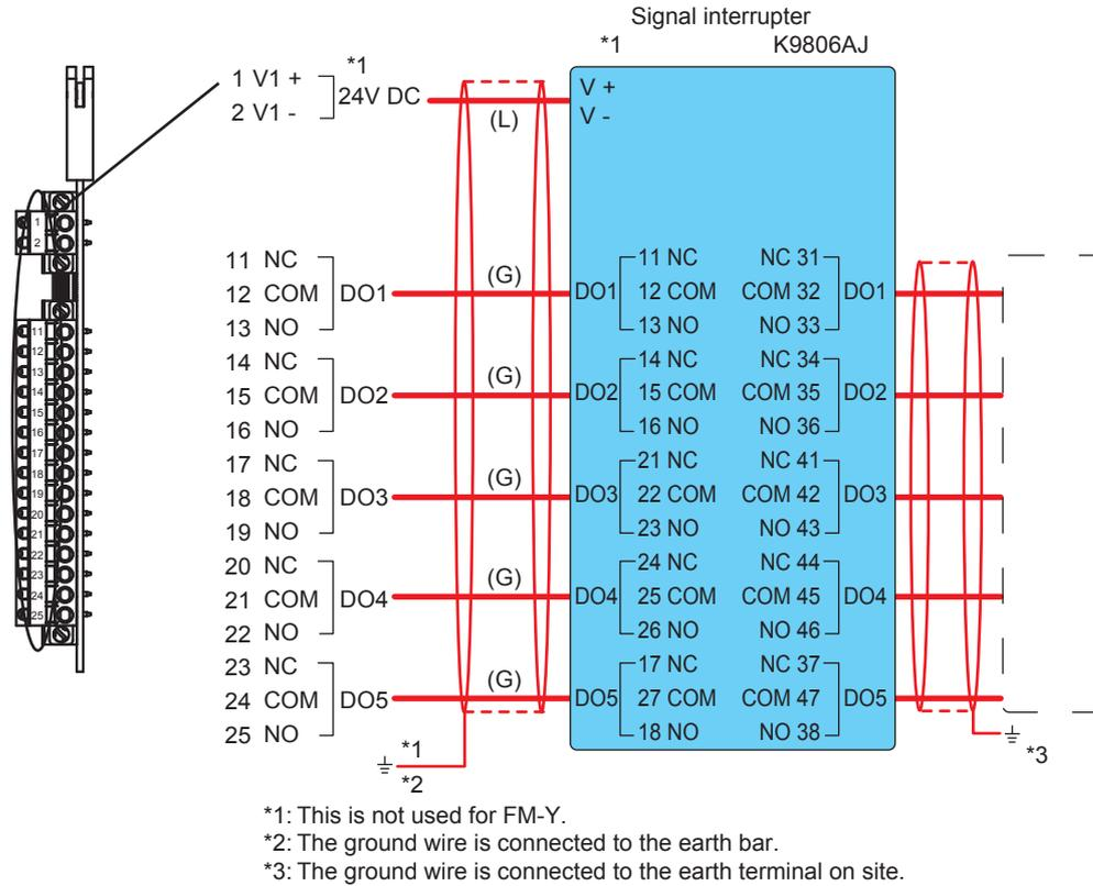
**Figure 2.31** Wiring for a contact output card
