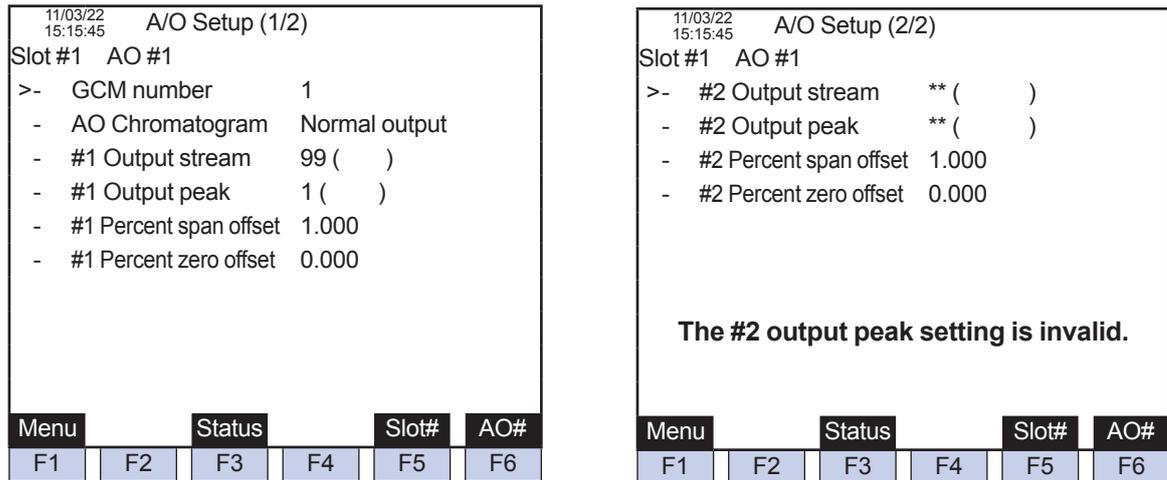
Figure 7 Analog Hold Output: Analysis Result of All the Streams that Belong to the GCM (AO Setting Screen on GC-HMI EtherLCD)
