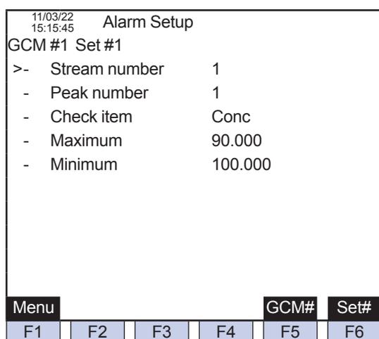
Figure 19 Alarm Setting Screen on GC-HMI EtherLCD
