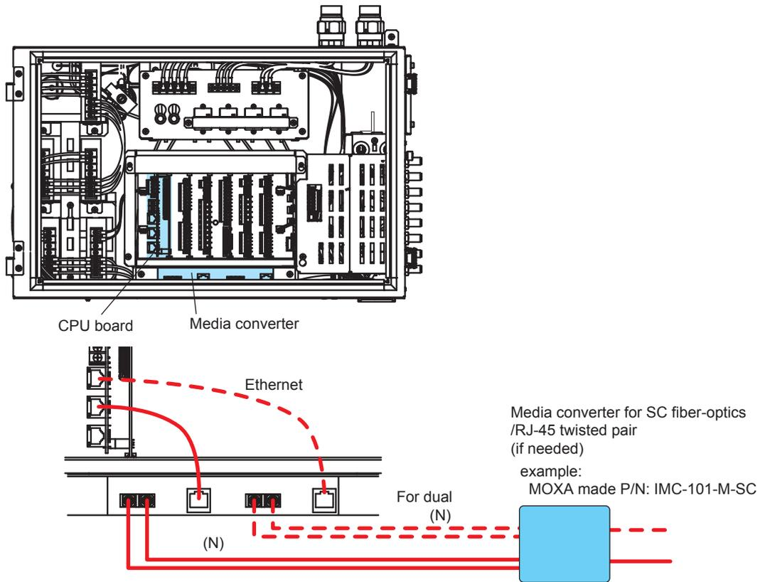
Figure 2.24 Ethernet (optical fiber)
