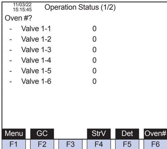
Figure 5.25 Example of the valve operation count screen (1/2)
