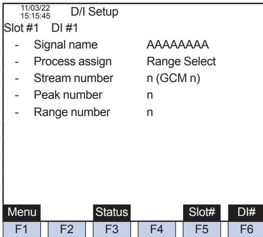
Figure 5.121 Example of DI setup screen (setting the Process assign to Range select)
