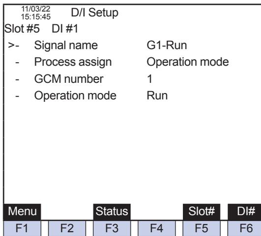
Figure 28 Process Specification: Operation Mode (DI Setting Screen on GC-HMI EtherLCD)
