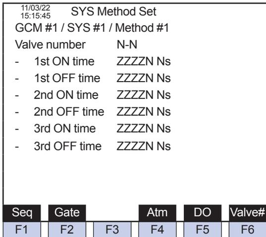
**Figure 5.86** Example of the SYS method setup (valve) screen
