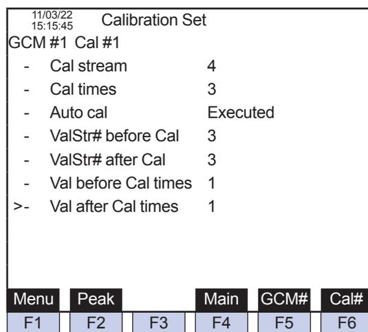
Figure 27 Calibration/Validation Setting Screen and Calibration Screen on GC-HMI EtherLCD.
