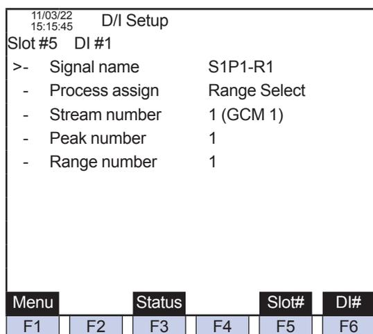
Figure 24 Process Specification: Range Switching (DI Setting Screen on GC-HMI EtherLCD)
