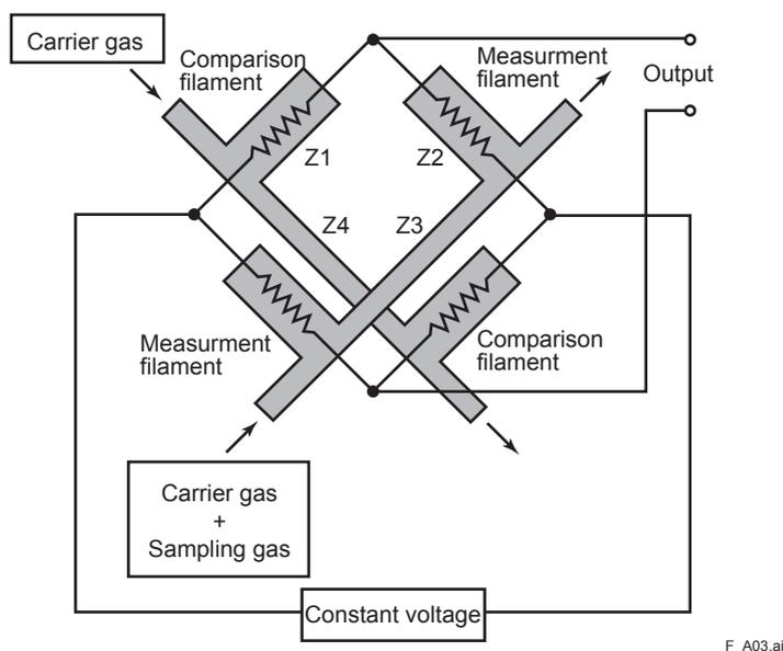
Figure 3 Fundamental Principle of Thermal Conductivity Detector
