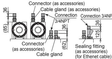
For ATEX (wiring connection: M25x1.5)
