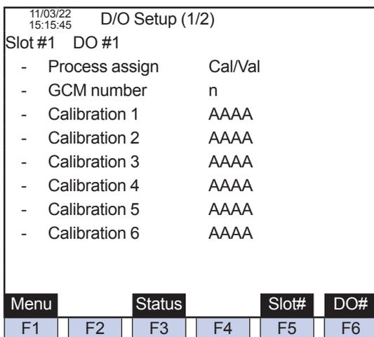
Figure 5.115 Example of DO setup (1/2) screen (setting the Process assign to Cal/Val)
