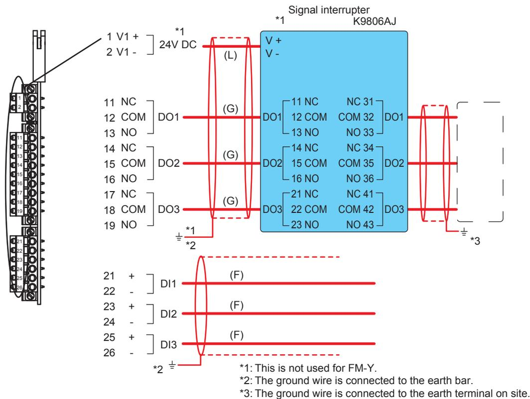
**Figure 2.34** Wiring for a contact input/output card
