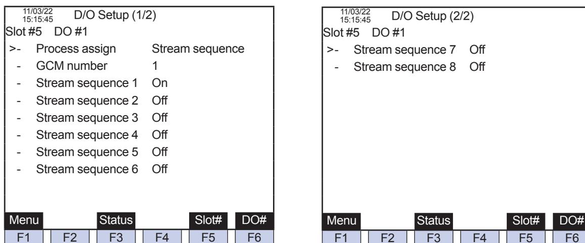
Figure 15 Process Specification: Stream Sequence (DO Setting Screen on GC-HMI EtherLCD)
