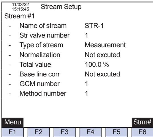
Figure 1.35 An example of the stream setting screen on the GC-HMI EtherLCD
