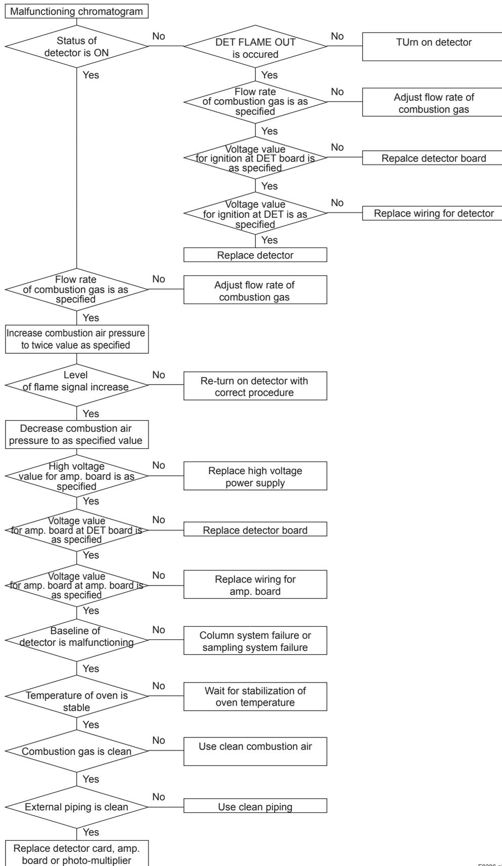
Figure 7.6 Troubleshooting Diagram for Malfunctioning Chromatogram (FPD)
