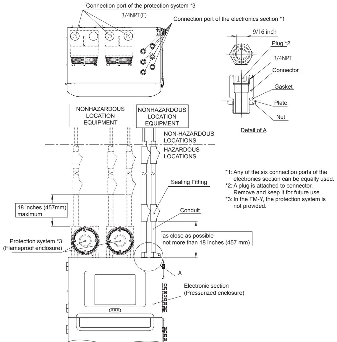
Figure 2.17 Wiring in FM specification
