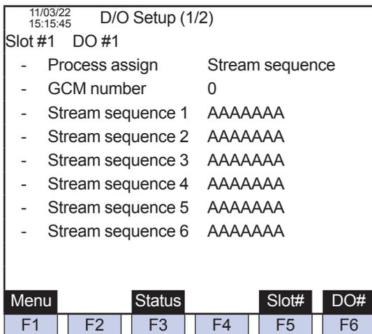
Figure 5.109 Example of DO setup (1/2) screen (setting the Process assign to stream sequence)
