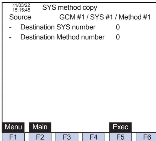
**Figure 5.81** Example of the SYS method copy screen
