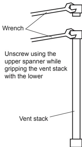
**Figure 2.3**      **Unscrewing the vent stack**
