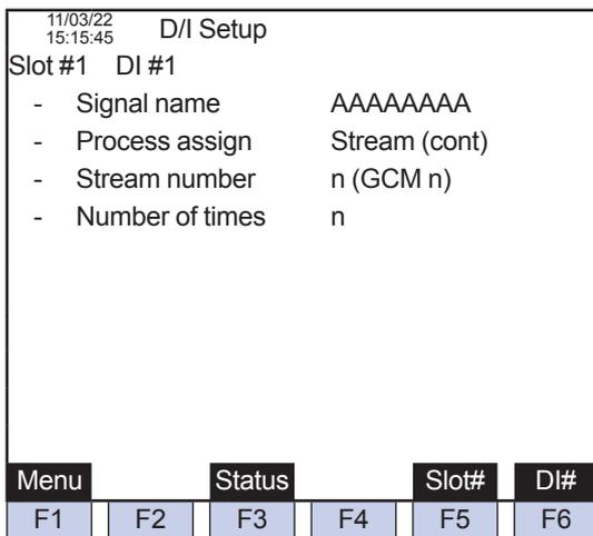
Figure 5.120 Example of DI setup (setting the Process assign to Stream)
