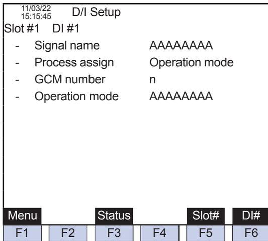
Figure 5.123 Example of DI setup screen (setting the Process assign to Operation mode)
