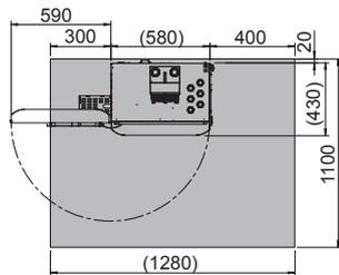
\*4: Required clearance needed for wiring.
