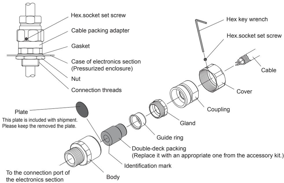
**Figure 2.14 Procedure for mounting a cable packing adapter for the electronics section**
