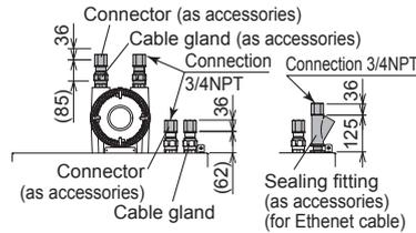
For ATEX (wiring connection: M25x1.5)
