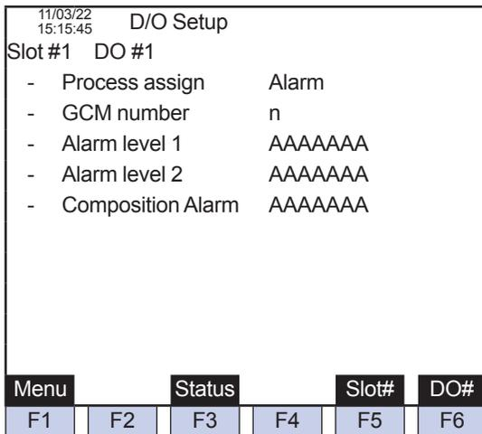
Figure 5.113 Example of DO setup screen (setting the Process assign to Alarm)
