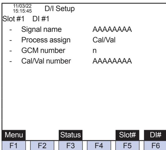
Figure 5.122 Example of DI setup screen (setting the Process assign to Cal (Val))
