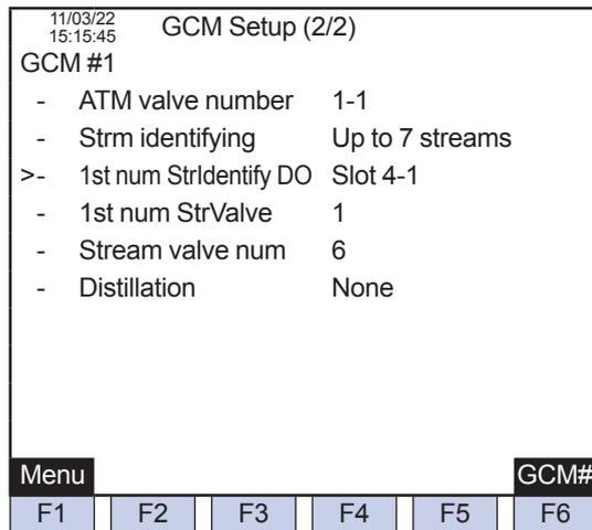
**Figure 4 Stream Identification Signal Output: Exist (GCM Setting Screen on GC-HMI EtherLCD)**
