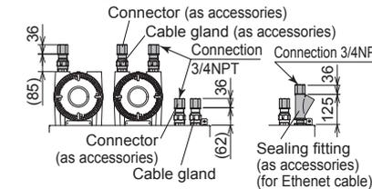
For ATEX (wiring connection: M25x1.5)
