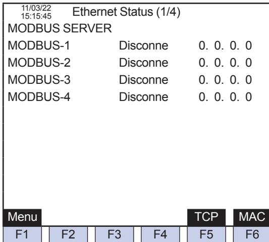
Figure 5.19 Modbus IP address screen (1/4)
