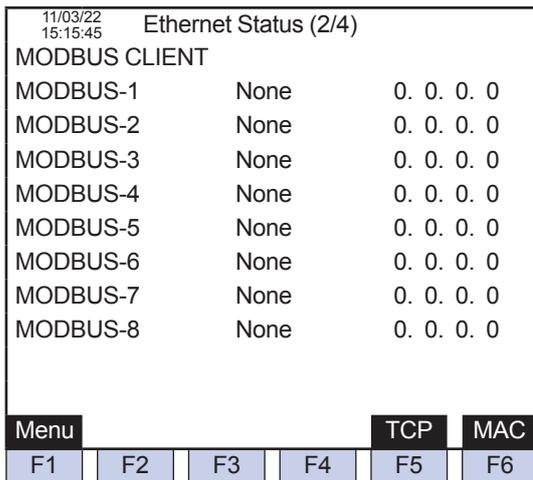
Figure 5.20 MODBUS IP address screen (2/4)
