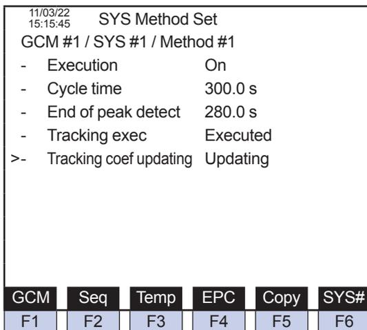
Figure 1.43 Tracking specification and automatic renewal of tracking factors in SYS method setting (GC-HMI EtherLCD)
