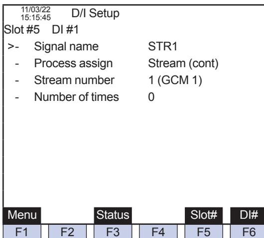
Figure 23 Process Specification: Stream (DI Setting Screen on GC-HMI EtherLCD)
