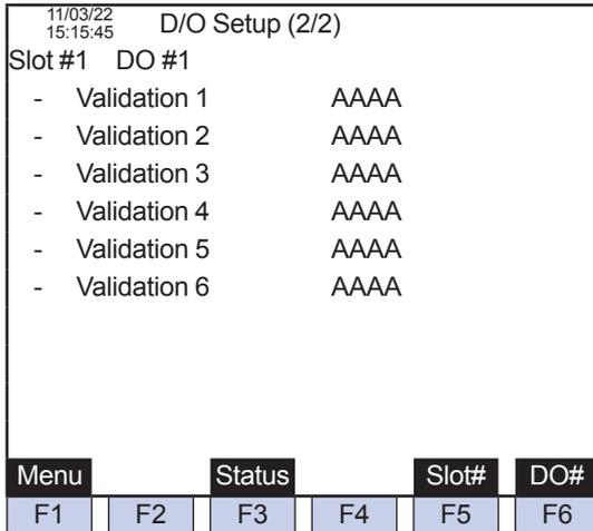
Figure 5.116 Example of DO setup (2/2) screen (setting the Process assign to Cal/Val)
