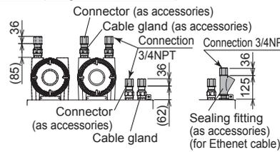
For ATEX (wiring connection: M25x1.5)
