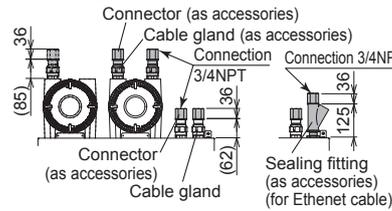
For ATEX (wiring connection: M25x1.5)
