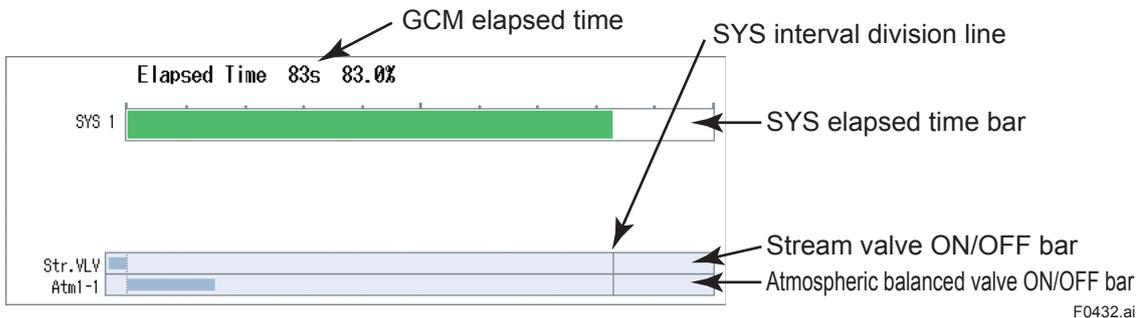
Figure 4.32 Display Example of Elapsed Time Bar
