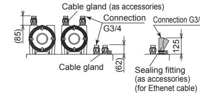
For FM-X (wiring connection: 3/4NPT)
