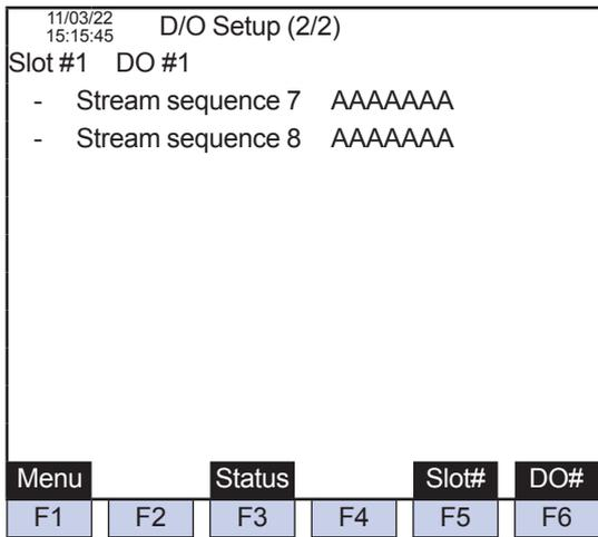
Figure 5.110 Example of DO setup (2/2 screen (setting the Process assign to stream sequence)
