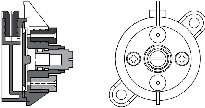
Figure 6.4 Pressure Switch for Detecting Internal Pressure
