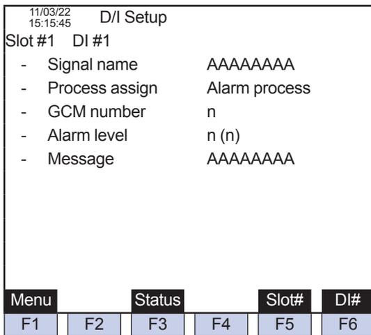
Figure 5.124 Example of DI setup screen (setting the Process assign to Alarm process)
