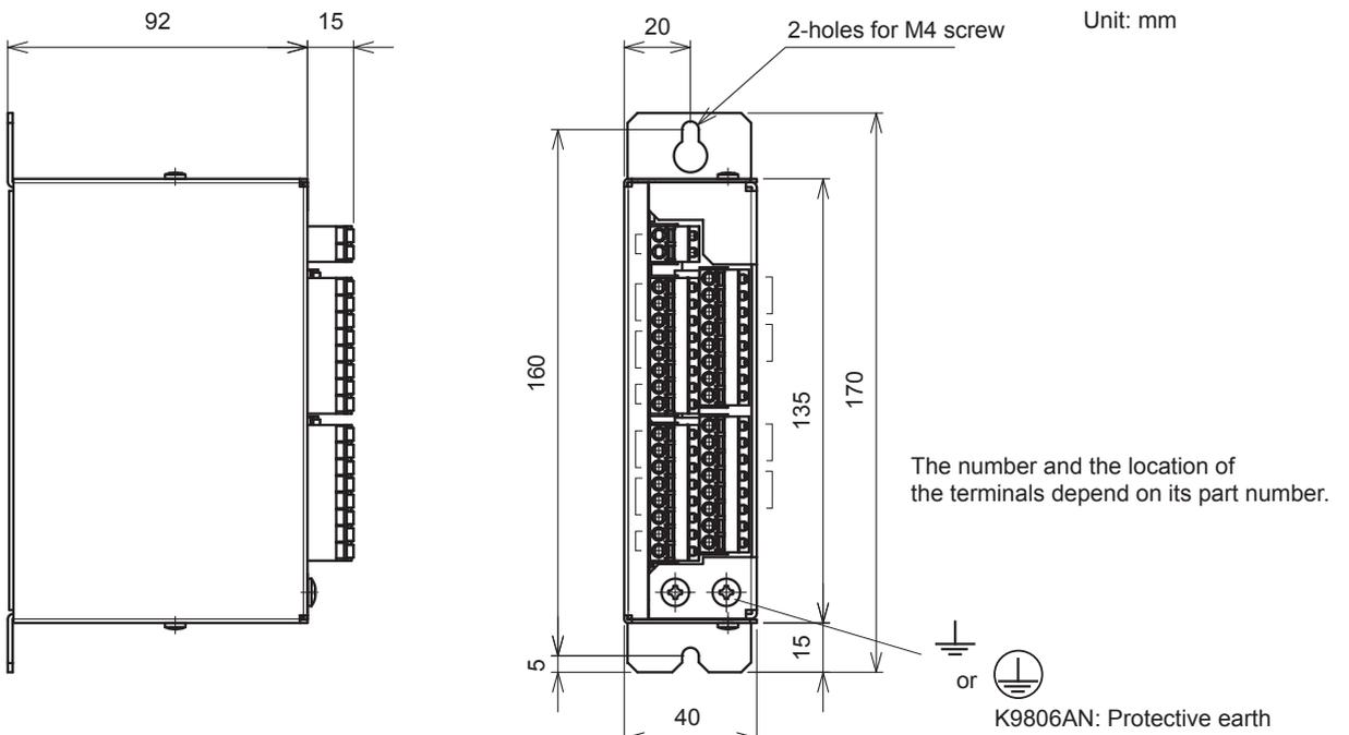
Note: Rack-mounted type should be installed vertically. The space between the converters/the signal interrupters with mark (\*) should be kept more than 10 mm.
