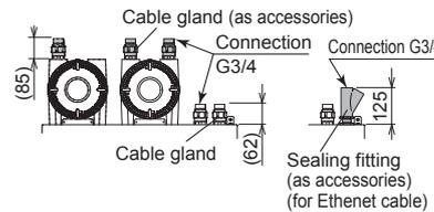
For FM-X (wiring connection: 3/4NPT)
