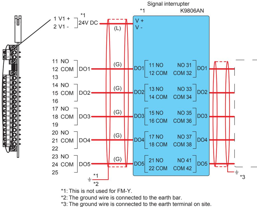
Figure 2.30 Wiring for a contact output card
