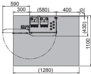
\*4: Required clearance needed for wiring.
