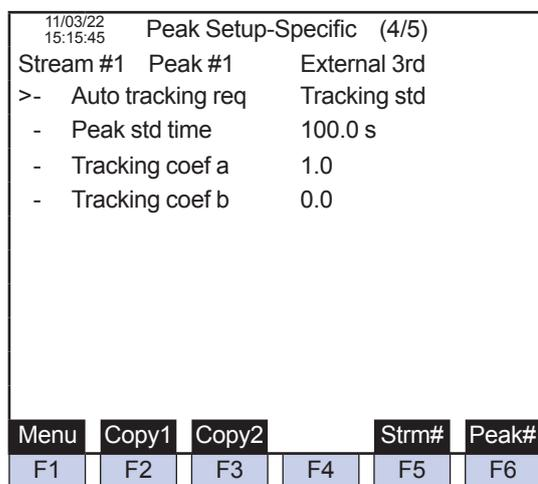
Figure 1.44 Tracking specification and tracking factor a/b in peak individual setting (GC-HMI EtherLCD)
