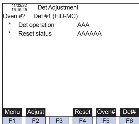
**Figure 5.55** Example of the detector type: FID-MC - reset screen
