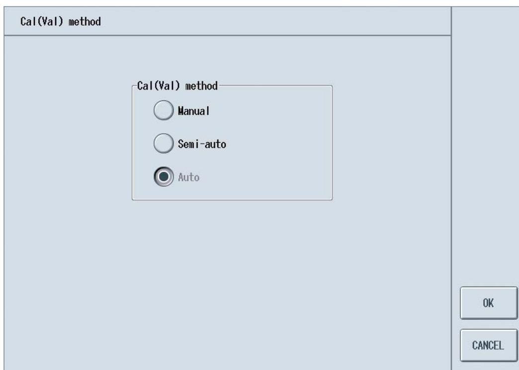
Figure 3.25 Calibration (validation) Method Setting Screen
