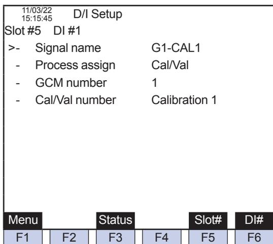
Figure 26 Process Specification: Calibration/Validation (DI Setting Screen on GC-HMI EtherLCD)
