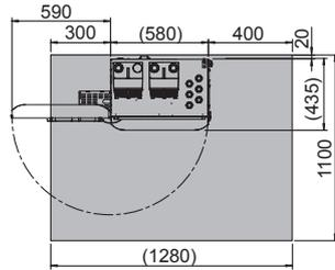
\*4: Required clearance needed for wiring.
