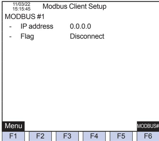
**Figure 5.144 Example of MODBUS Client Setup screen**
