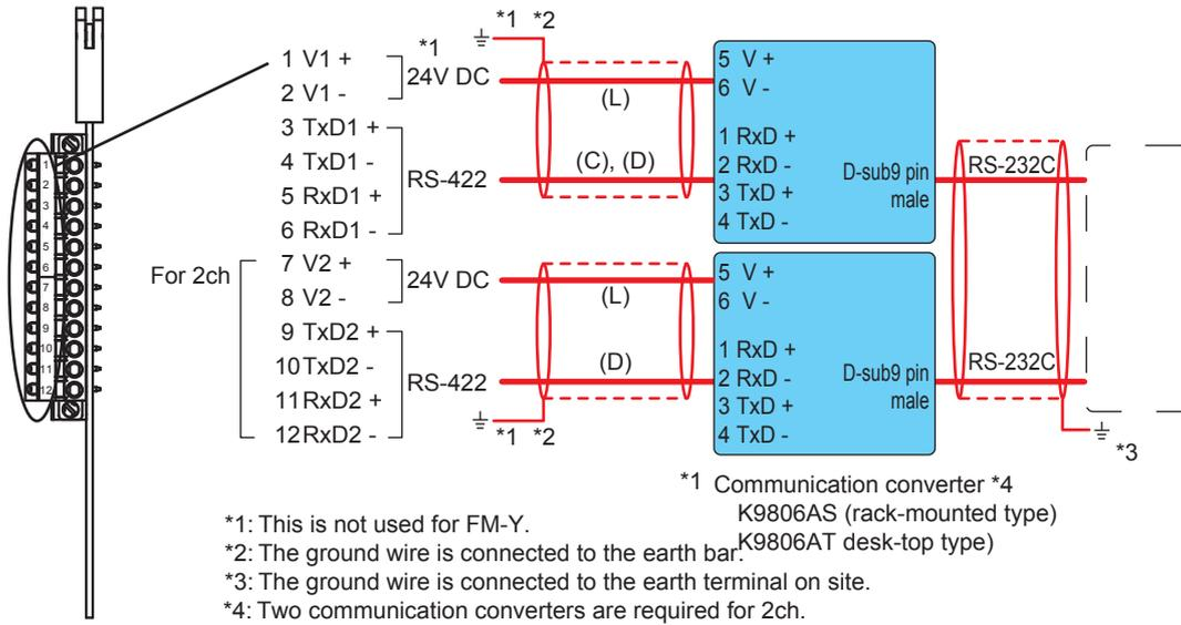
Figure 2.27 Wiring for serial communication cards
