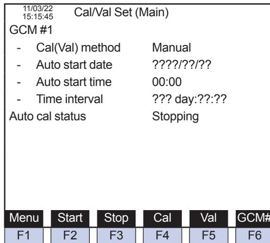
**Figure 5.96** Example of Cal/Val Set (main) screen
