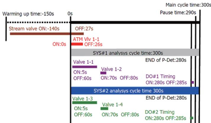
Figure 1.37 GCM method and SYS method setting example 1
