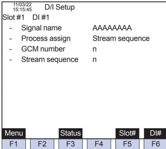
Figure 5.119 Example of DI setup screen (setting the Process assign to Stream sequence)
