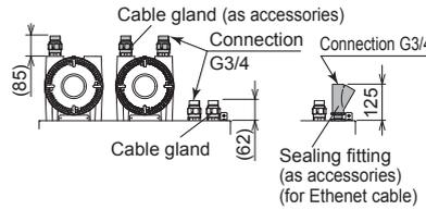
For FM-X (wiring connection: 3/4NPT)
