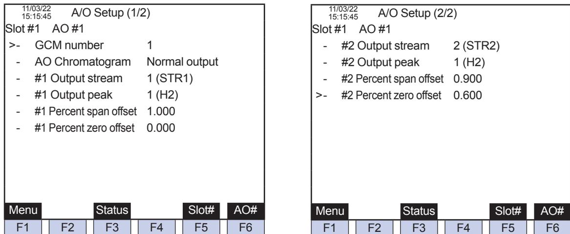
**Figure 1 Analog Hold Output: Analysis Result of Actual Streams (AO Setting Screen on GC-HMI EtherLCD)**
