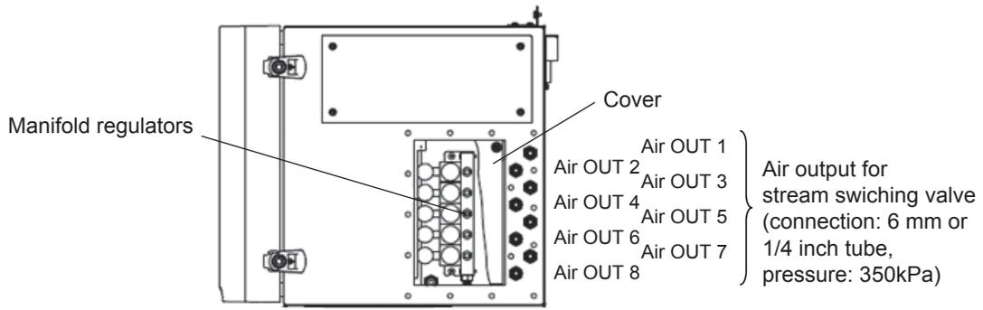
Figure 1.6 Pressure control section of the control unit
