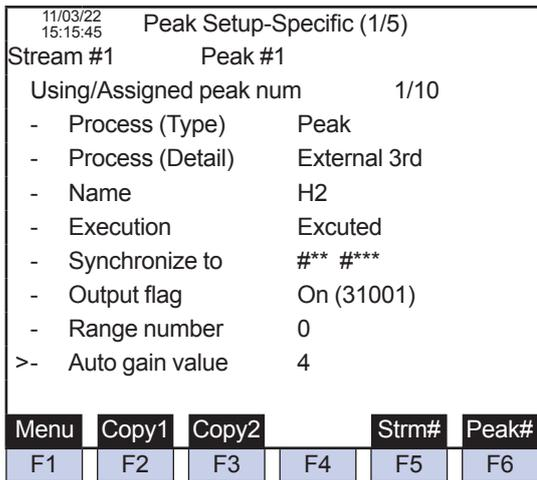
Figure 11 Auto Gain Value (Individual Peak Setting Screen on GC-HMI EtherLCD)
