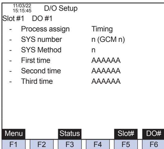
Figure 5.114 Example of DO setup screen (setting the Process assign to Timing)
