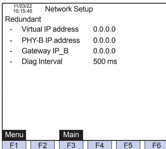
Figure 5.129 Example of network setup (Redundant) screen
