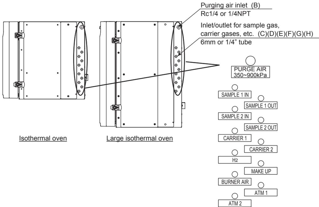
Figure 2.7 Left side of isothermal oven and large isothermal oven
