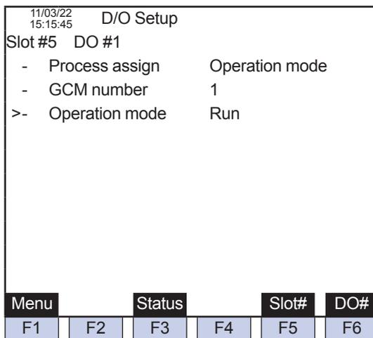
Figure 17 Process Specification: Operation Mode (DO Setting Screen on GC-HMI EtherLCD)
