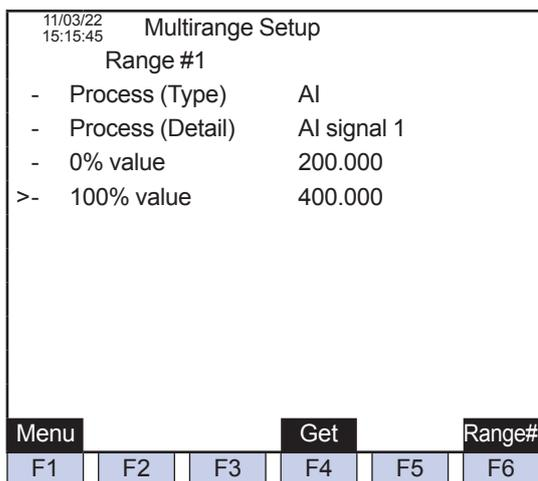
Figure 13 AI Processing (Multi-Range Setting Screen on GC-HMI EtherLCD)
