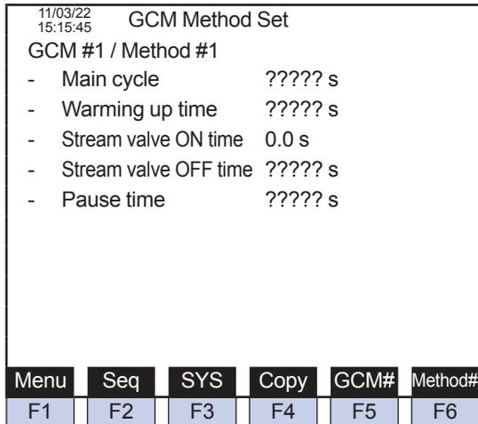
Figure 5.76 Example of the GCM method setup screen
