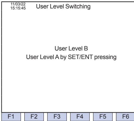
**Figure 5.3** Example of the user level switching screen (when the current level is other than A)
