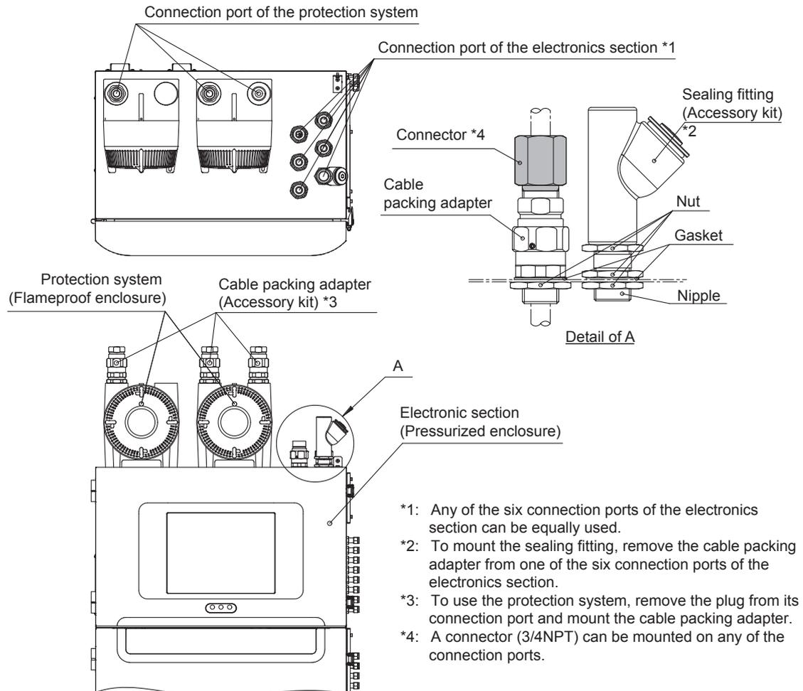
Figure 2.12 Wiring in TIIS specification
