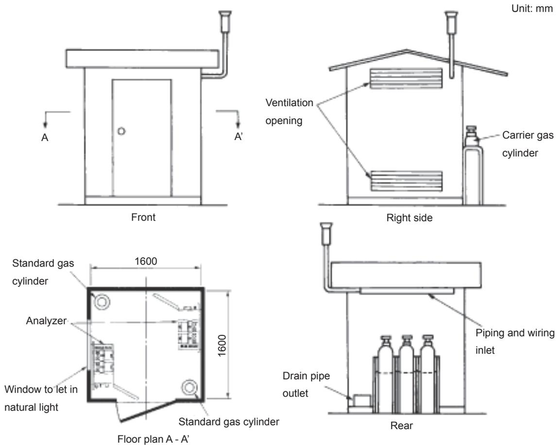
Figure 2.1 Example of analyzer house
