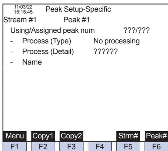
Figure 5.93 Example of peak setup-specific screen (when process assignment is not processed).
