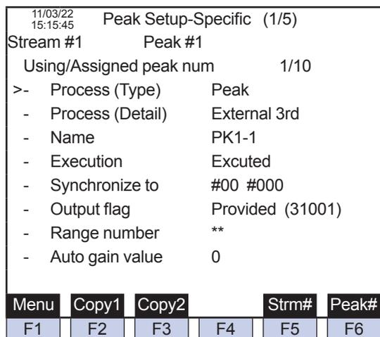
Figure 3.23 Example of calibration peak setting screen
