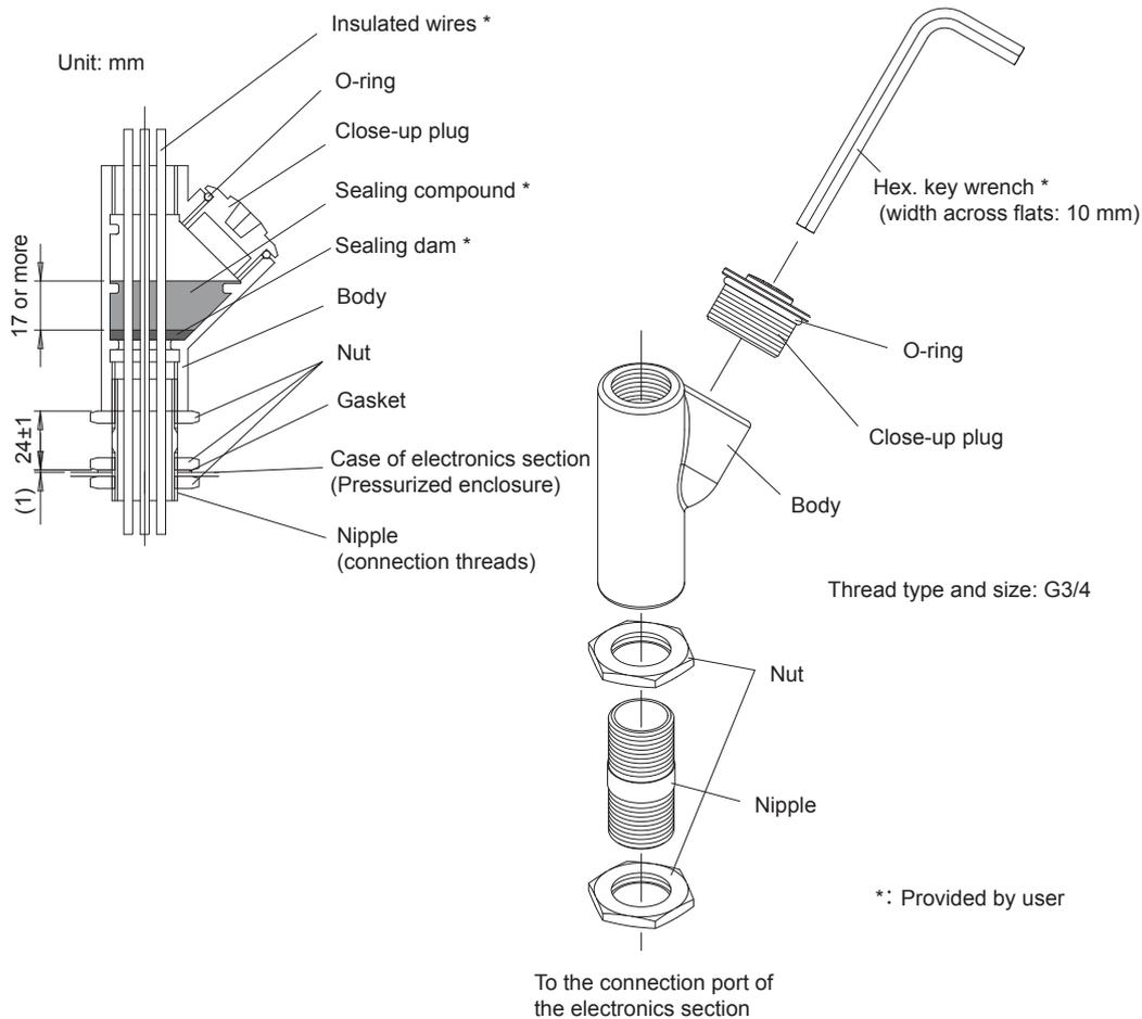
Figure 2.15 Mounting procedure for sealing fitting (accessory)
