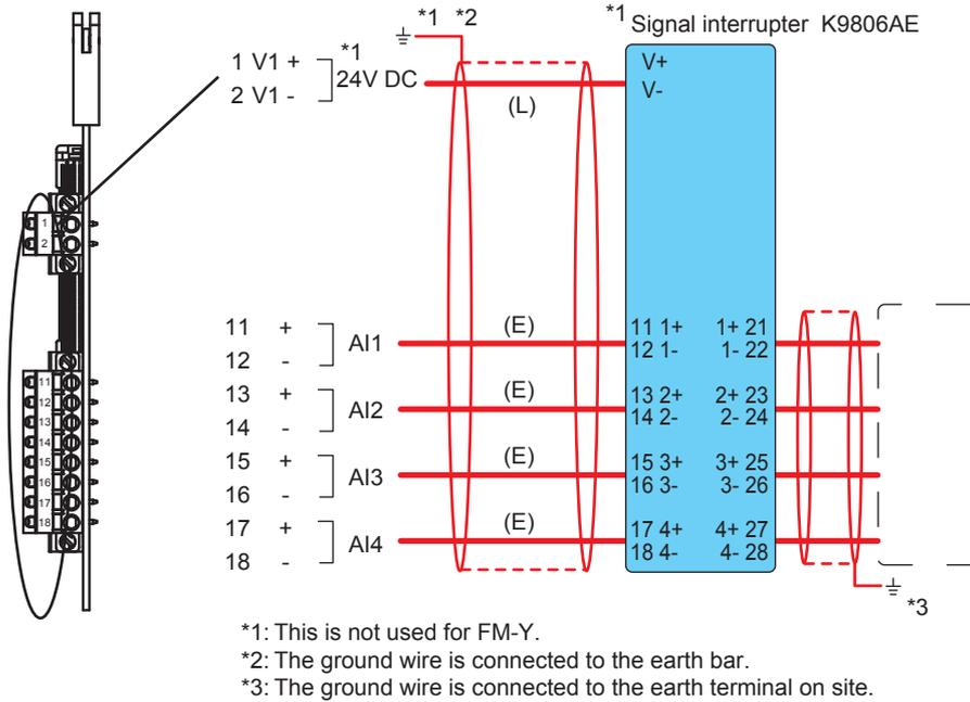
Figure 2.29 Wiring for an analog input card
