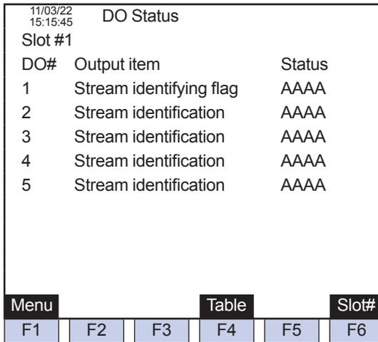
**Figure 5.10 Example of the DO Status screen (Stream Identification)**
