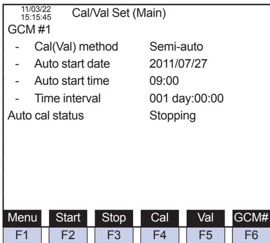
Figure 1.29 An example of the calibration/validation setting screen on the GC-HMI EtherLCD.
