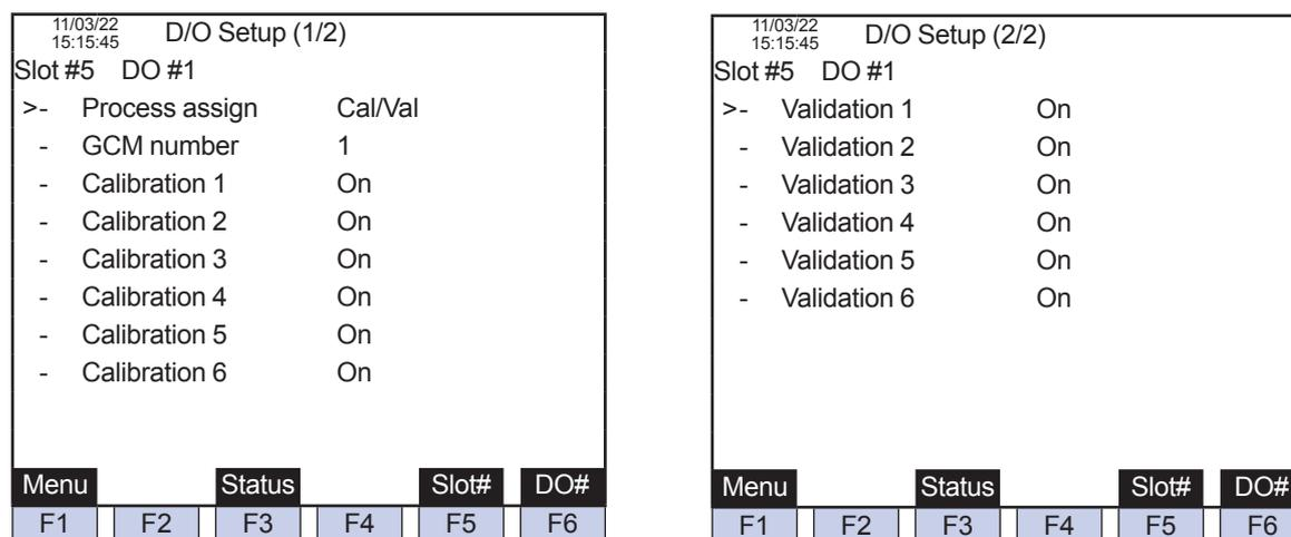
Figure 20 Process Specification: Calibration/Validation (DO Setting Screen on GC-HMI EtherLCD)
