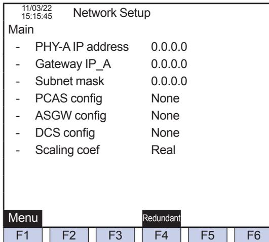
Figure 5.128 Example of network setup (Main) screen
