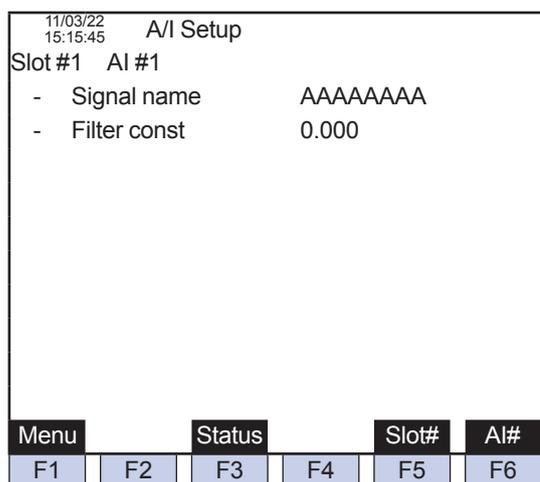
**Figure 5.127 Example of AI setup screen**
