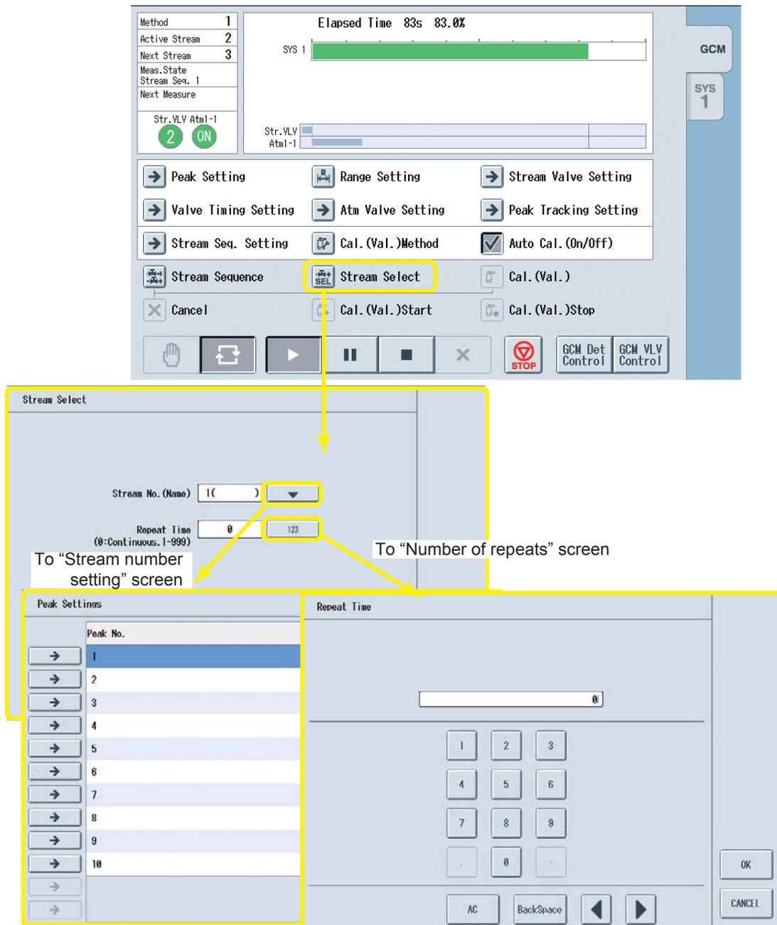
Figure 1.22 An example of the stream specification window on the GCM operation status screen on the GC-HMI analyzer operation display
