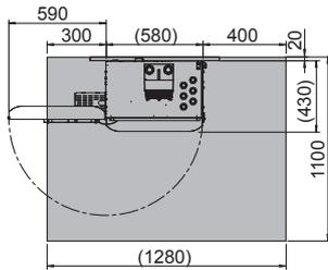
\*4: Required clearance needed for wiring.
