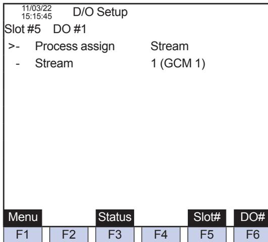
Figure 16 Process Specification: Stream (DO Setting Screen on GC-HMI EtherLCD)
