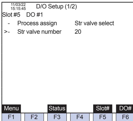
Figure 21 Process Specification: Stream Valve Switching (DO Setting Screen on GC-HMI EtherLCD)
