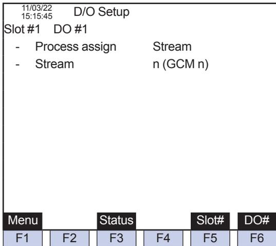
Figure 5.111 Example of DO setup screen (setting the Process assign to stream)
