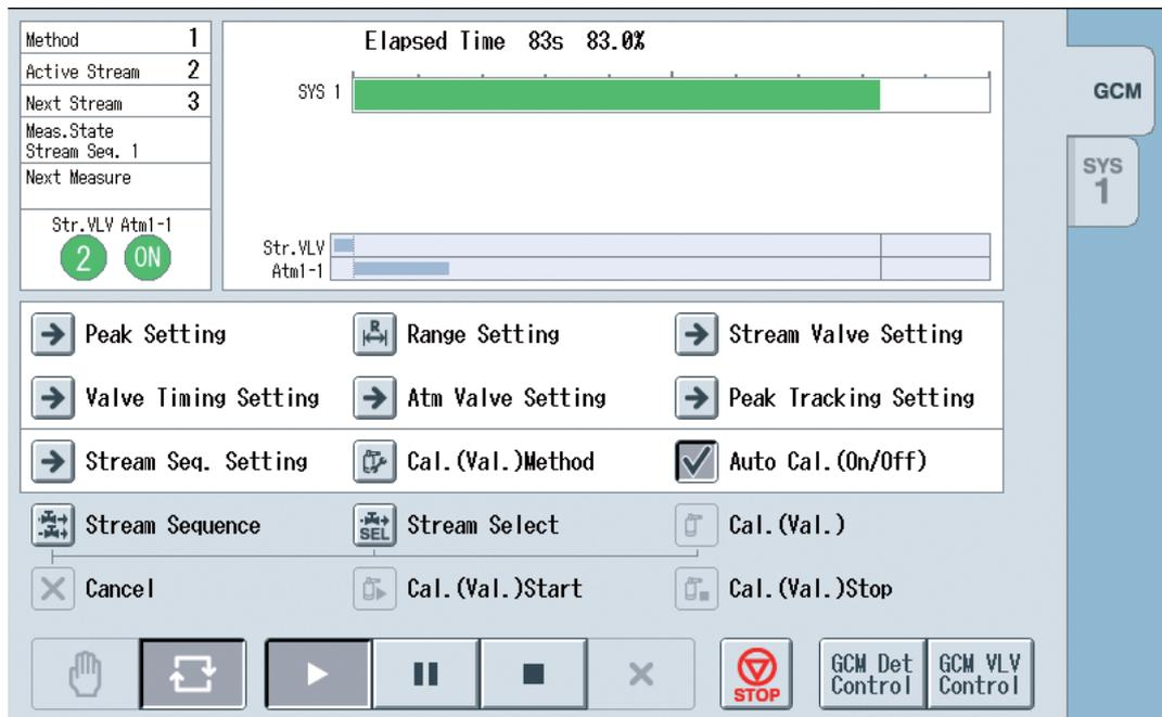
Figure 1.17 Analyzer Operation screen of the GC-HMI (touch panel)
