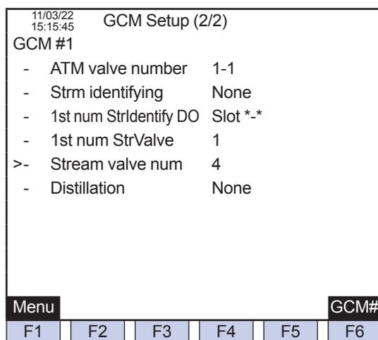
**Figure 2 Stream Identification Signal Output: None (GCM Setting Screen on GC-HMI EtherLCD)**
