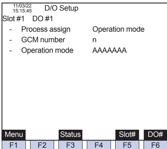
Figure 5.112 Example of DO setup screen (setting the Process assign to Operation mode)
