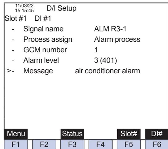
Figure 29 Process Specification: Alarm Setting (DI Setting Screen on GC-HMI EtherLCD)
