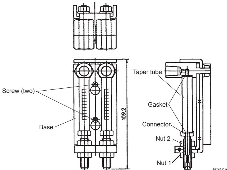
**Figure 6.47 Taper Tube**
