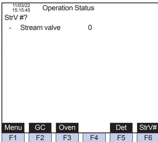
**Figure 5.27** Example of the operation status screen (Stream Valve Operation Count)
