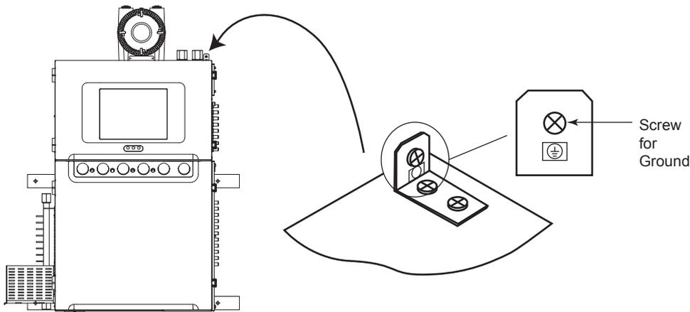
Figure 2.21 Earth terminal for the GC8000
