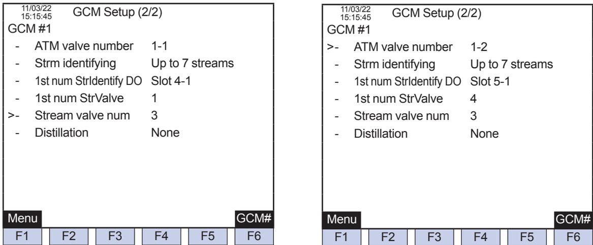
Figure 5 Stream Identification Signal Output: Exist (GCM Setting Screen on GC-HMI EtherLCD)
