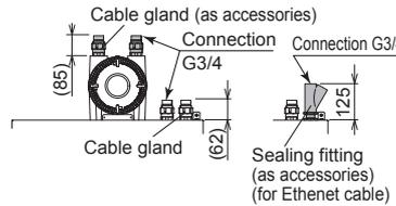
For FM-X (wiring connection: 3/4NPT)
