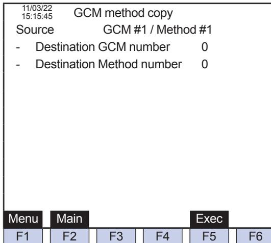
**Figure 5.77** Example of the GCM method copy screen
