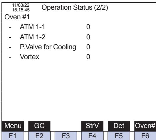
Figure 5.26 Example of the valve operation count screen (2/2)
