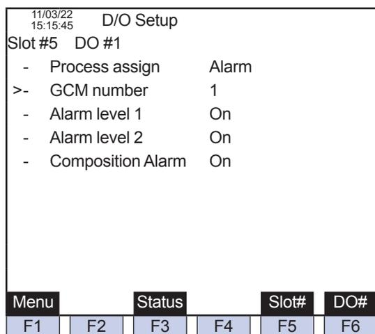
Figure 18 Process Specification: Alarm (DO Setting Screen on GC-HMI EtherLCD)
