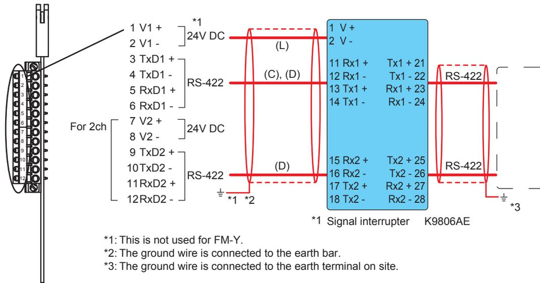
Figure2.26 Wiring for serial communication cards
