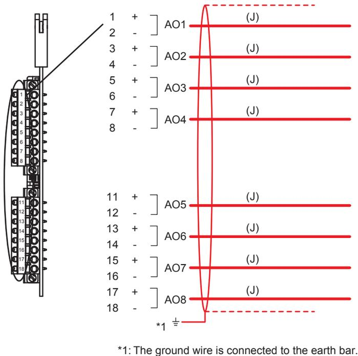
Figure 2.28 Wiring for an analog output card
