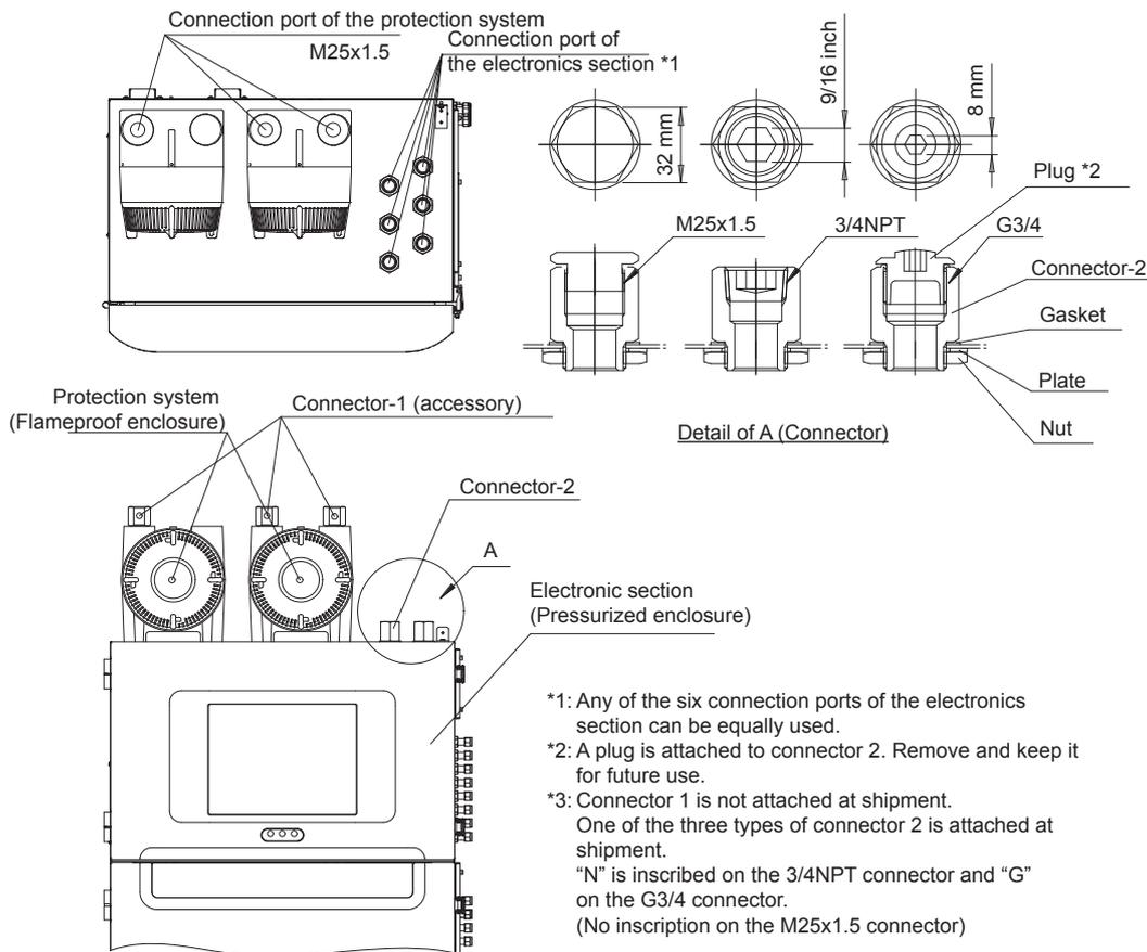
Figure 2.16 Wiring in ATEX specification
