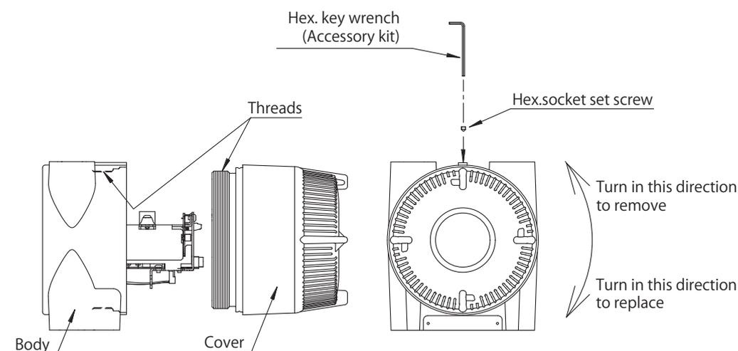
**Figure4 Opening/closing the cover of the protection system**
