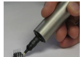
Figure 1: IC Pin Voltage Measurement
